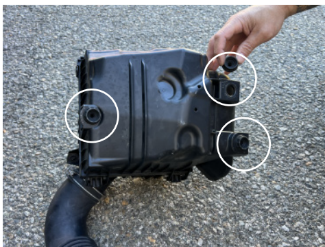
7. Remove the (3) three factory mounting grommets from factory air box.
