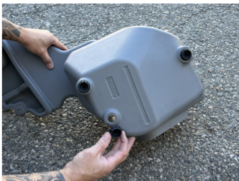
8. Install the (3) three factory mounting grommets onto EVO2203 air box.
