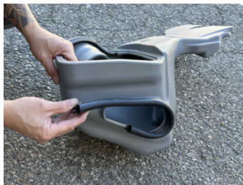
9. Install rubber bulb trim onto passenger side fender opening on EVO2203 air box.
