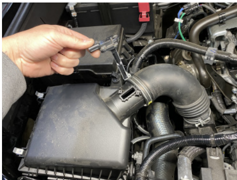
4. Unbolt MAF and remove from factory intake.
