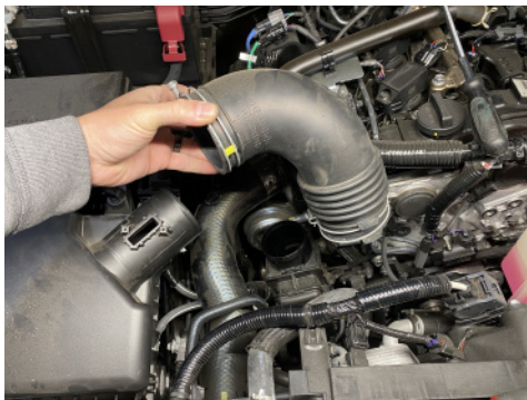
5. Loosen clamps and remove factory intake tube.
