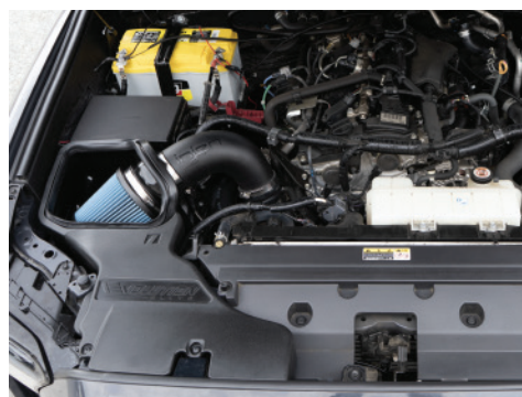
18. Secure intake tube to both turbo inlet hose and air box hose.
