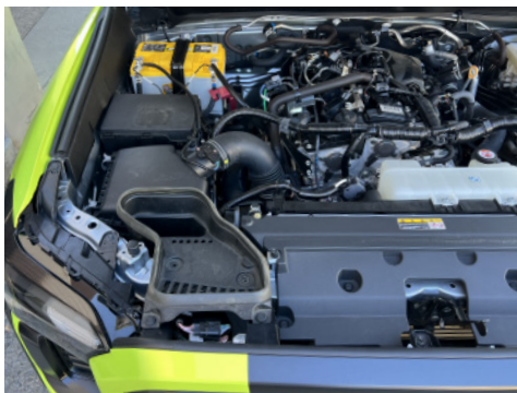
1. Factory intake system.
