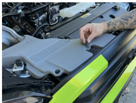
12. Using provided push pins, secure air box to radiator support.
