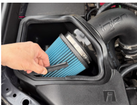
20. Install provided rubber trim onto air box as shown and trim accordingly.
