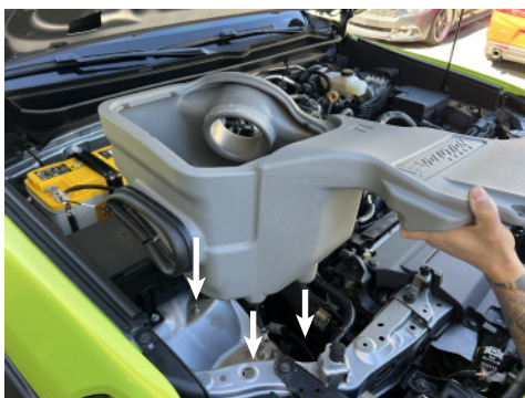
10. Align mounting grommets on EVO2203 air box to factory mounting studs.
