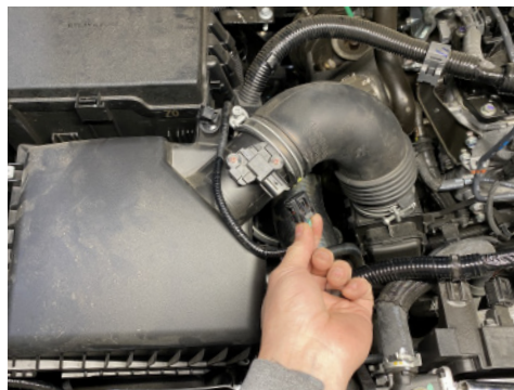
3. Disconnect MAF sensor connector.
