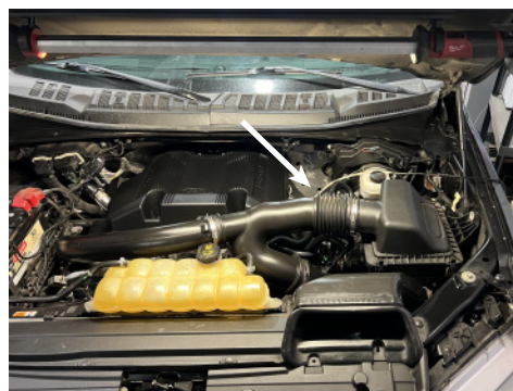
23a. Locate the air temperature sensor and harness. If the lead comes from the REAR of the engine, refer to PAGE 5.
