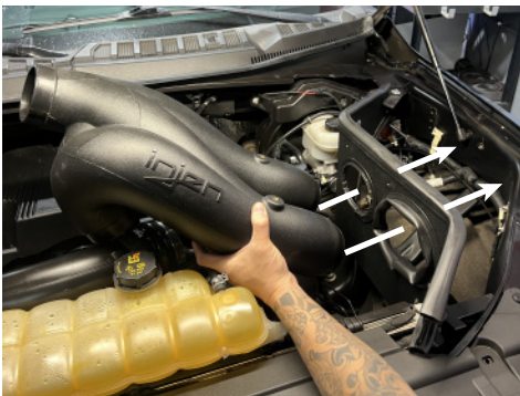
27b. Install mounting bracket onto vibramounts on heat shield using provided hardware and secure.
