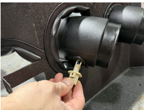
33b. Install air temp sensor into the front of the intake tube and secure.
