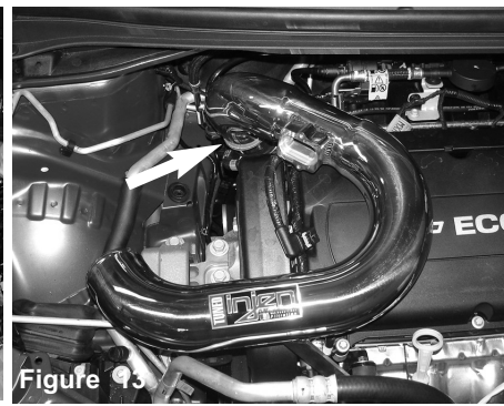
Figure 10 Locate the black bracket left of the oil dip stick. Place the Vibramount with a washer and M6 nut to secure it to the bracket
