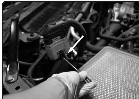
10. Using a flat head screwdriver, carefully unclip the ECU harness from the lower part of the air box. Do not Disconnect harness!
