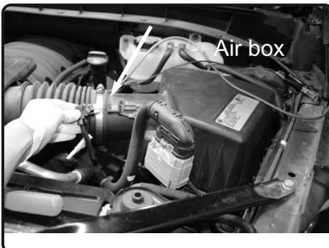
5. Disconnect the MAF sensor harness.
