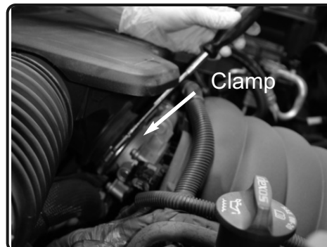
7. Loosen the clamp on the throttle body using 8mm nut driver.
