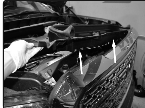
3. Remove the push clips, and carefully remove the plastic radiator shroud.
