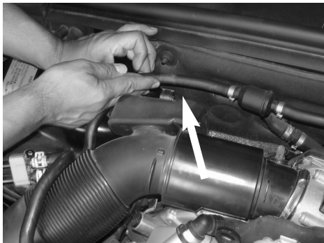
Figure 6 Pull back the vacuum line from the intake tube.
