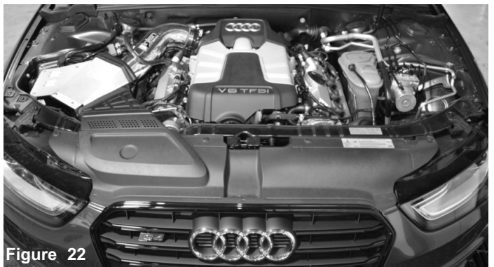
Figure 20 Install the engine cover to the top of the air box, and secure using provided coarse screws and tighten using T25 torx screw driver.
