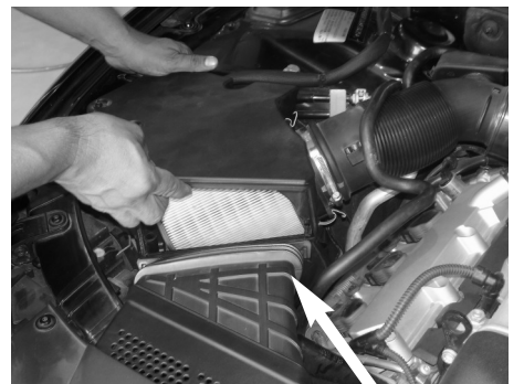
Figure 8 With all lines pulled away from the stock intake system, lift up and remove the stock intake system.
