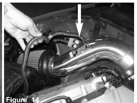
Figure 14 Install the intake tube and position the intake system to the throttle body hose.
