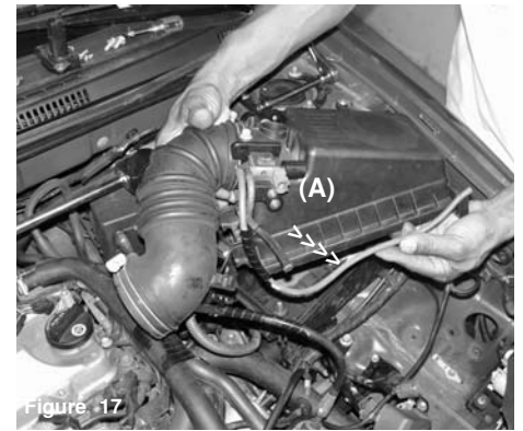
Figure 17 The line that was disconnected from the butterfly valve(VAD) is held to one side (A). The entire top air box cleaner is now removed the the lower air box.
