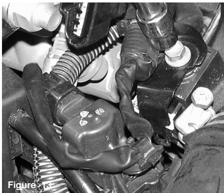
Figure 13 Loosen and remove the PWM vacuum switching valve bolt with a 10 mm socket and ratchet as shown above.
