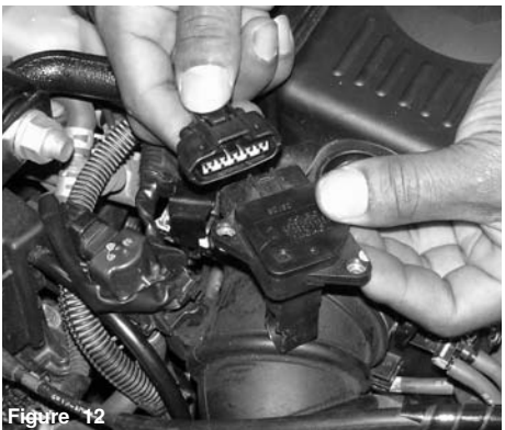
Figure 12 As you remove the mass air flow sensor, unclip the electrical sensor harness as shown above.
