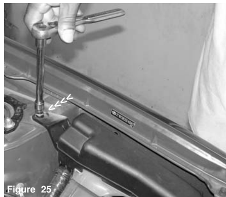
Figure 25 Loosen and remove the m6 nut from the fuse box located on the strut tower mount.
