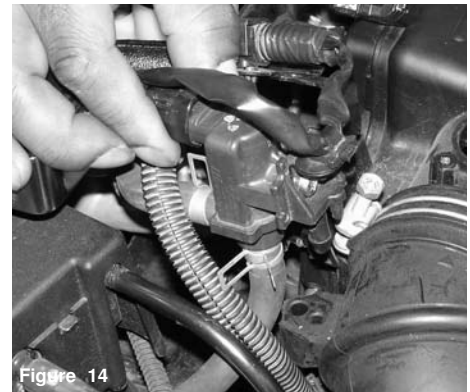
Figure 14 Once you have removed the m6 bolt, continue to pull the VSV from the rubber air duct cradle.
