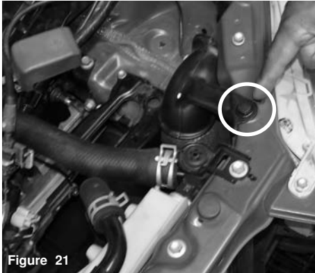
Figure 21 Pull the plastic clip up and remove the clip from the cross member, this will release the air resonator air duct.
