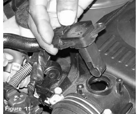
Figure 11 Once you have removed the two screws, continue to remove the mass air flow sensor from the sensor housing.
