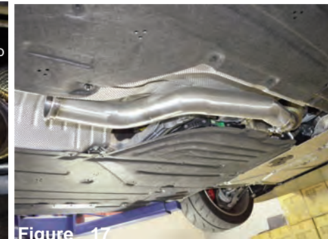
Figure 17 Adjust and set into position. Do not tighten. Note: Exhaust system has room for adjustment, re-position and tighten for best fit.
