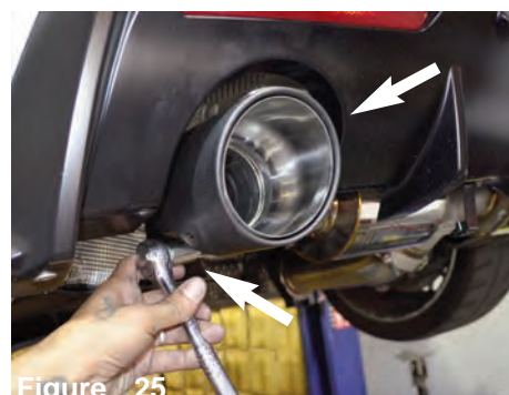
Figure 25 Now install the carbon fiber tips to the rear muffler assembly. Secure and tighten and adjust to desired position.
