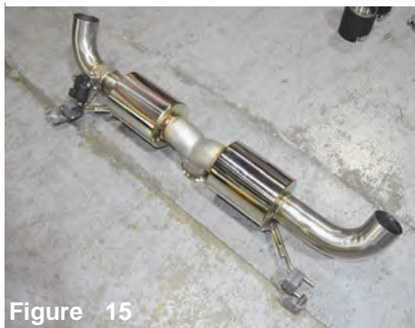
Figure 15 Re-install the hangars to the injen rear muffler assembly.
