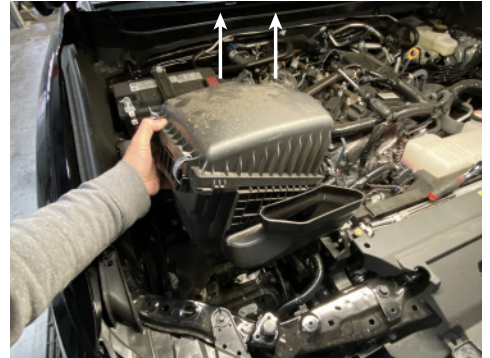
6. Remove factory air box by applying some force while pulling up on assembly.
