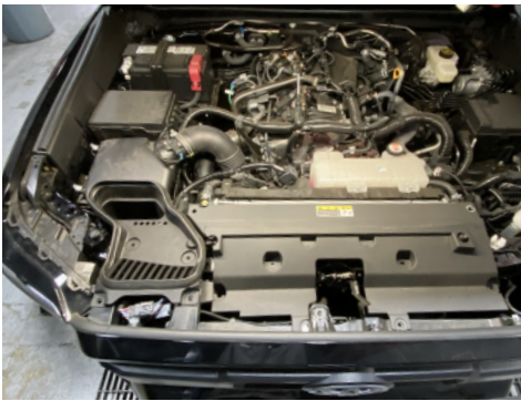
1. Factory intake system.
