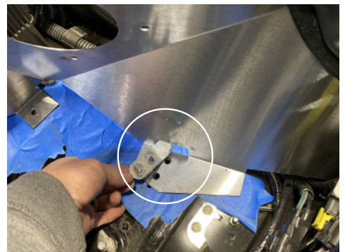
12. Feed chassis ground through opening at the bottom of the heat shield.
