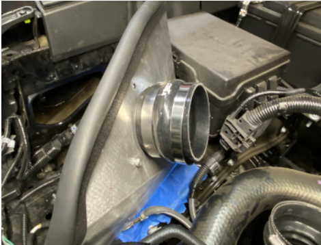
16. Install 3.75" hump hose to velocity stack/heat shield assembly and secure hose clamp.
