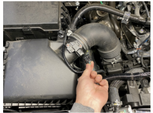
3. Disconnect MAF sensor connector.
