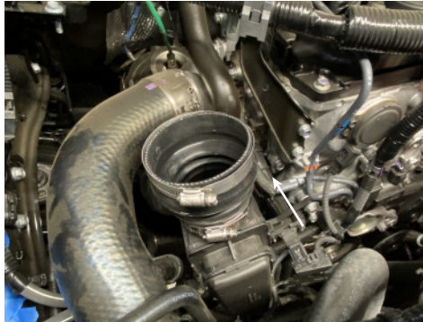
17. Install 3.50"-2.75" stepped double hump hose to turbo inlet and secure hose clamp.
