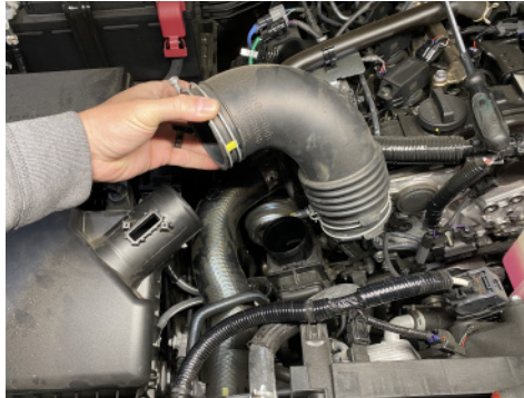
5. Loosen clamps and remove factory intake tube.
