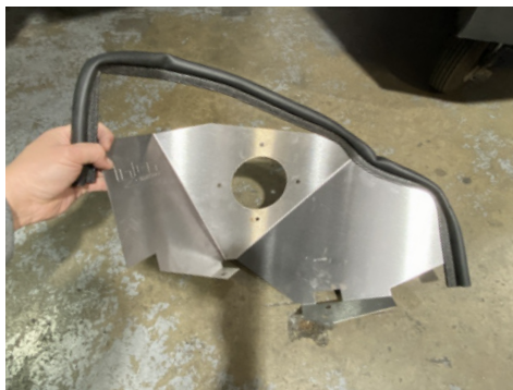
11. Install provided rubber bulb trim to heat shield. Trim excess material as needed.
