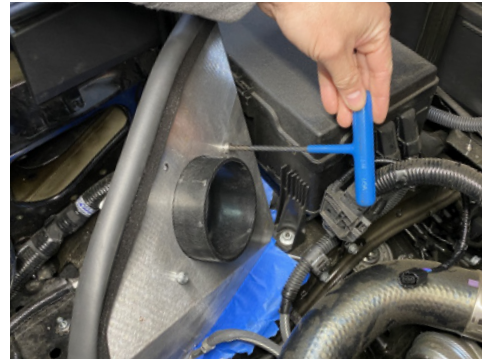
15. Bolt velocity stack to heat shield using the (4) provided 12mm hex bolts through intake tube side of heat shield.
