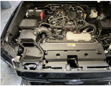
1. Factory intake system.
