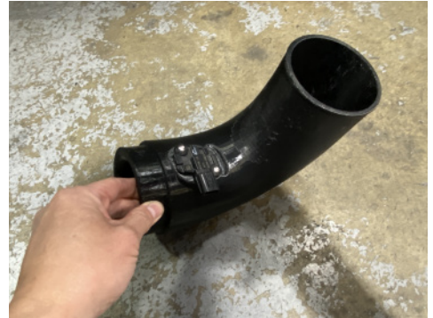
18. Install and secure MAF sensor to PF2013 intake tube using the (2) button head screws provided.
