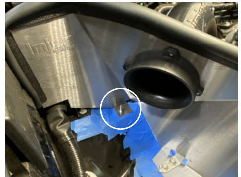
21. Bolt factory upper mounting stud (saved from figure 8) to heat shield.
