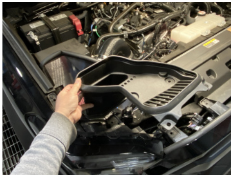
23. Reinstall factory air scoop.
