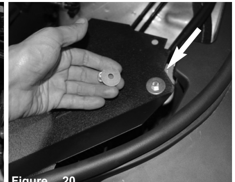
Figure 20 Secure the heatshield using provided M6 screw fender washers and M6 lock nut.
