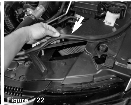
Figure 22 Attach the green tree push pin on the trim seal into the hole on the heatshield scoop inlet.
