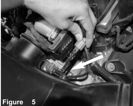
Figure 5 Disconnect the Temperature sensor and remove the sensor from the intake tube.
