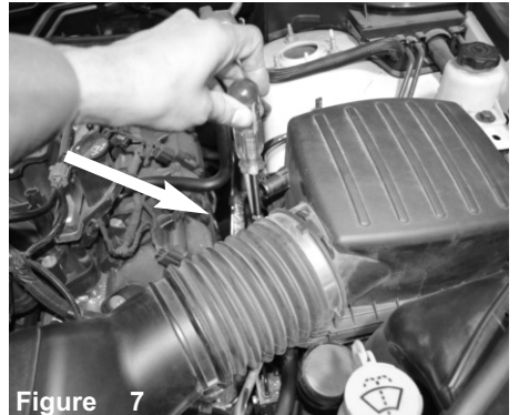
Figure 7 Loosen the clamp on the air box.
