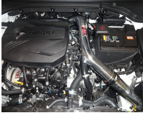
29. Ensure all clamps and nuts are properly secured. Once complete reinstall the front bumper.
