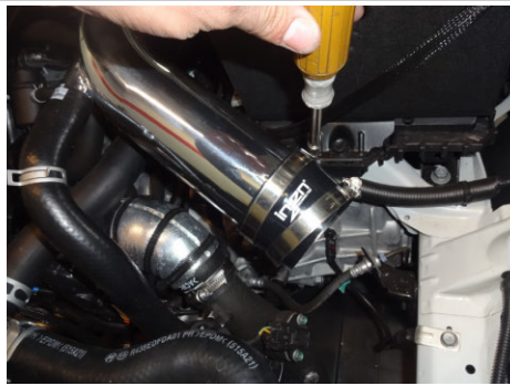
20. Place the 3.0" straight hose and two clamps onto the intake tube. Only secure the clamp on the intake side for now.
