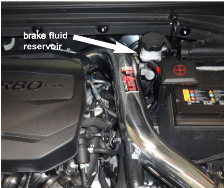
16. CAUTION: Make sure the intake pipe has adequate clearance from the brake fluid reservoir. Adjust the intake pipe for best possible fitment and then secure the all the clamps.
