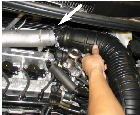
5. Loosen the clamp on the that is securing the intake tube to the turbo inlet. Detach the intake tube from the turbo inlet.
