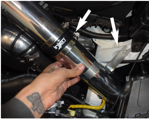
25. Insert the secondary tube into the 3.0" straight hose, then line up the bracket to the vibra mount.
