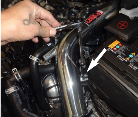
13. Secure the intake bracket to the vibra mount using the provide M6 nut and washer.
