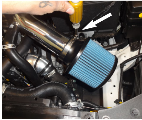
17. If installing the cold air intake, proceed to step 19. Place the filter onto the end of the intake pipe and then secure the clamp on the filter.
