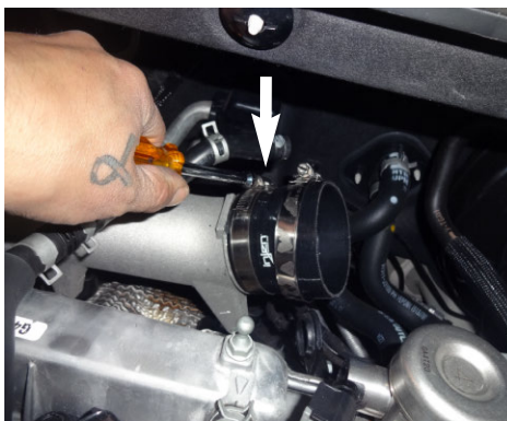
10. Place the 2.75"-3.00" step hose onto the turbo inlet. Only secure the clamp on turbo inlet for now.
