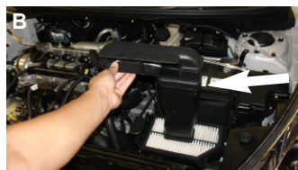
8. Figure A: Remove the two plastic clips from the front air intake duct. Figure B: Lift up and remove the front air intake duct.
