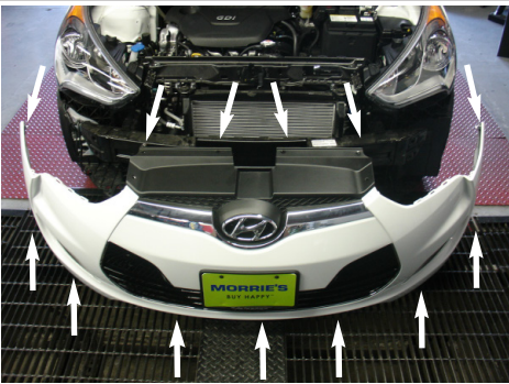
19. To continue with the installation of the cold air intake system, you will have to remove the front bumper cover by removing all the plastic retaining clips and screws indicated by the arrows in the photo.
