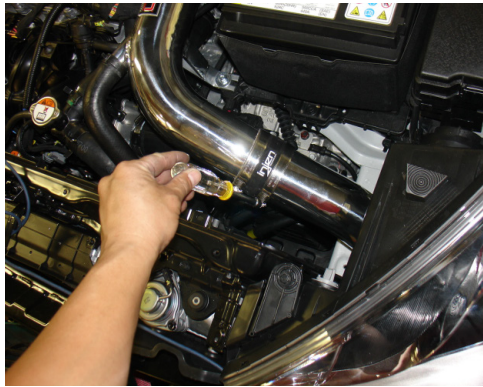
26. Reattach the primary intake tube to the turbo inlet hose, then ensure both brackets line up to their respective vibra mount. Once both tubes are lined up properly, secure both clamps on the 3.0" hose
