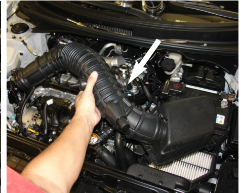
6. Remove the entire upper air box assembly from the engine bay.
