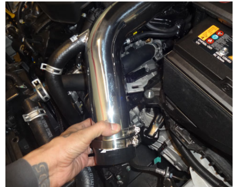
24. For easier installation, detach the upper intake from the vibra mount and turbo inlet hose. Next, route the Injen secondary intake pipe through the bumper cavity into the engine bay.
