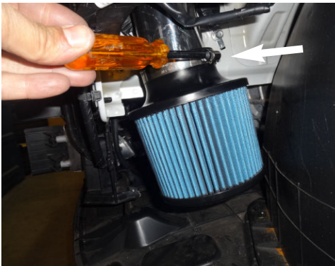
28. Place the filter onto the end of the intake pipe, then secure the clamp on the filter.
