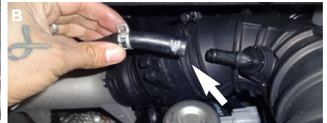
3. Figure A: Disconnect the recirculating diverter valve hose from the intake tube. Figure B: Disconnect the crank case breather line from the intake tube.
