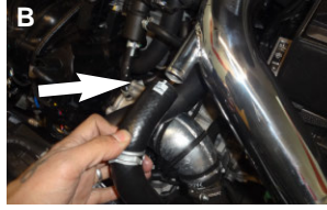
14. Figure A: Connect the crank case breather line to the 0.5" nipple on the intake pipe. Figure B: Connect the recirculating diverter valve hose onto the 1.0" nipple onto the intake pipe
