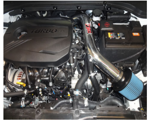
18. Reinstall the engine cover. Ensure all nuts and bolts are secured. Congratulations, your short ram intake system installation is now complete.
