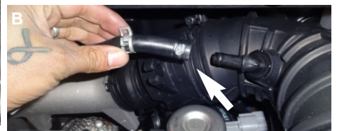
3. Figure A: Disconnect the recirculating diverter valve hose from the intake tube. Figure B: Disconnect the crank case breather line from the intake tube.
