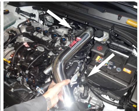
12. Install the intake tube. Insert the tube into the step hose then line up the bracket to the vibra mount.
