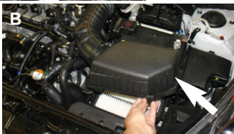
4. Figure A: Unclip the two tabs from the lower air box assembly to the upper air box assembly. Figure B: Detach the upper air box assembly from the lower assembly.
