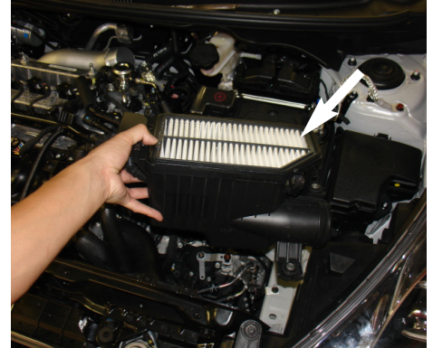
9. Remove the lower air box assembly from the engine bay.
