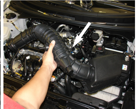
6. Remove the entire upper air box assembly from the engine bay.
