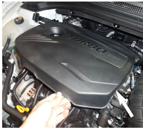
2. Firmly lift up on the engine cover and remove the engine cover from the engine bay.
