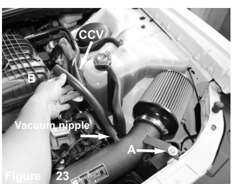
Figure 23 (A) Use a M6 nut and fender washer to secure the intake bracket to the vibramount. Make your final adjustment and secure the clamp on the hose in figure 5 (B) Use the 10"-15mm vacuum hose and connect the vacuum nipple on the intake tube to the crank case vent tube
