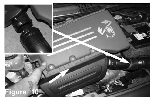
Figure 10 Now lift up and remove the air-box/engine cover from the vehicle. Disconnect the snorkel from the air box assembly.
