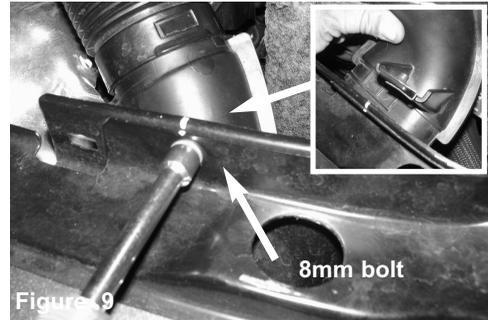
Figure 9 Loosen the bolt holding in the snorkel scoop on the radiator support. Now pull back the snorkel scoop from the radiator support.
