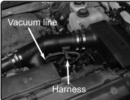
**15.** Connect the vacuum line to the 3/8" barbed fitting if equipped and then connect the MAF sensor harness to the MAF sensor.
