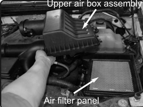
2. Disconnect the MAF sensor harness and unclip the 3 metal tabs holding the upper air box to the lower air box. Remove the upper box assembly and air filter panel.
