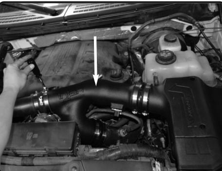
**14.** Install the Injen intake tube and connect all the couplers and secure the intake tube by tightening the clamps once its been adjusted.
