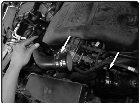
**13.** Place a 4.00" humpse and 2-#64 clamps onto the 4.00" OE inlet tube and the 3.50"-3.25" step hose and #48 & # 56 clamp onto the 3.25" OE inlet tube.
