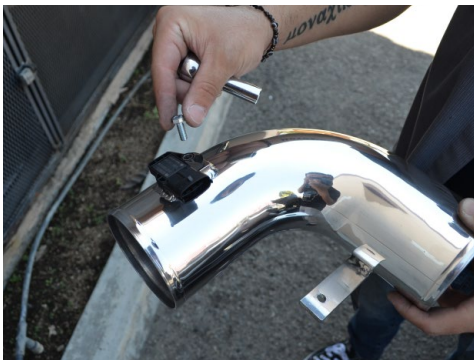
16. Install the IAT sensor onto the injen tube, then secure using the provided M6X15MM hex bolt.
