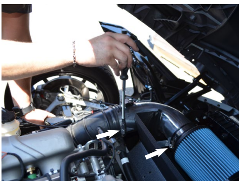
19. Install the air filter onto the intake tube, then secure the filter clamp and the OEM hose clamp.
