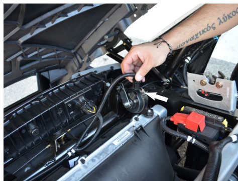
9. Disconnect the car horn harness.
