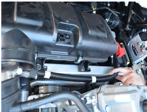
5. Detach the harness from the air box.
