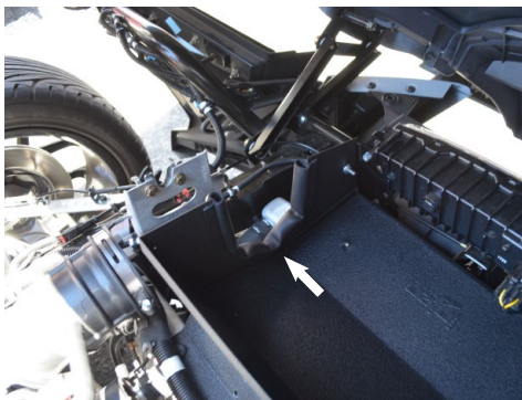
14. Install the bulb trim onto the heatshield.
