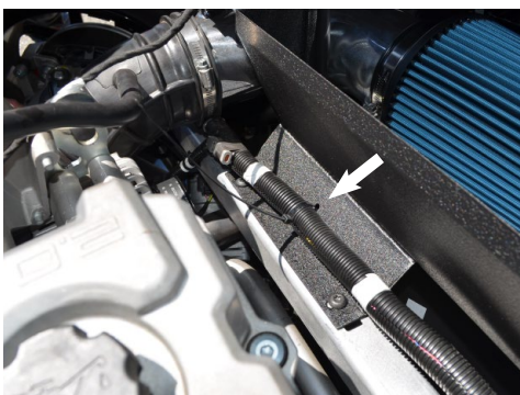
22. Run the zip tie through the two holes on the heat shield and secure the harness to the heat shield.
