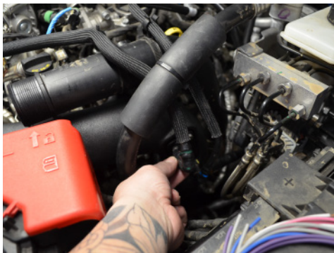
40. Reconnect both crankcase lines to the crankcase adapter.
