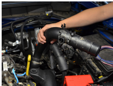
39. Reinstall the driver side charge pipe.
