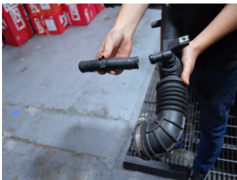
44. Remove the diverter valve hose from the OEM intake tube.
