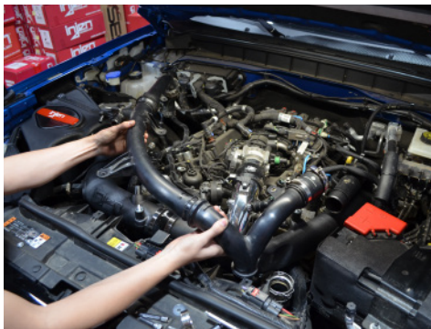
41. Reinstall the charge pipe.
