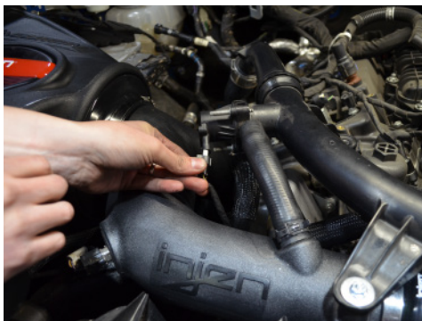
46. Reconnect the diverter valve harness.
