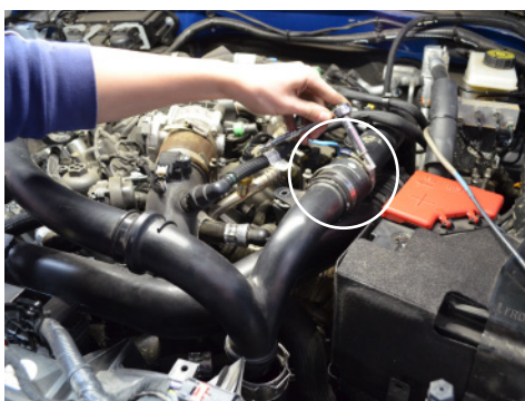
7. Loosen the clamp connecting the driver side charge pipe and the Y connecting pipe then remove the charge pipe.
