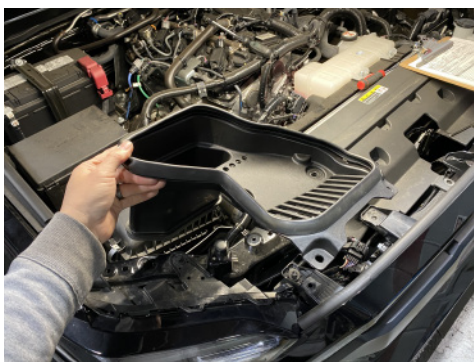
2. Remove factory air scoop.
