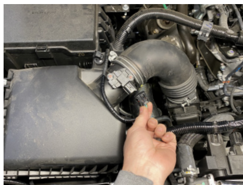
3. Disconnect MAF sensor connector.
