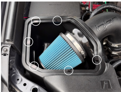
21b. Locate the (6) metal clips on the air box.
