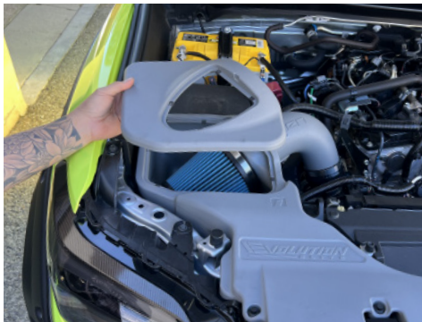
21a. Align lid to air box and install.
