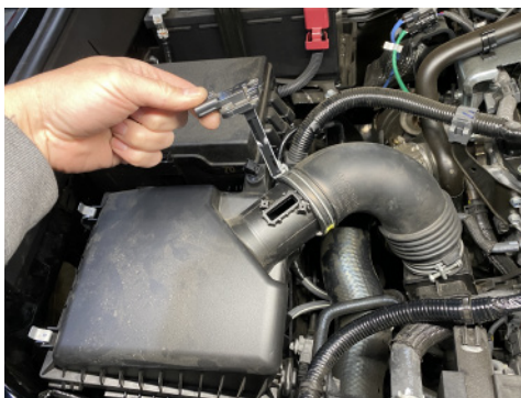
4. Unbolt MAF and remove from factory intake.
