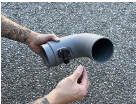
13. Install and secure MAF sensor to EVO2201 intake tube using the (2) two button head screws provided.
