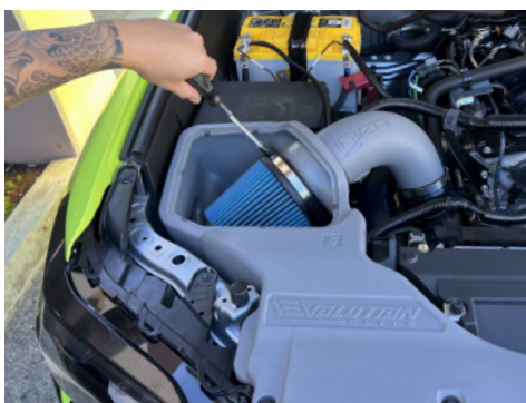
19. Install air filter and secure to air box.
