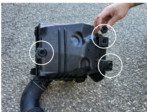
7. Remove the (3) three factory mounting grommets from factory air box.
