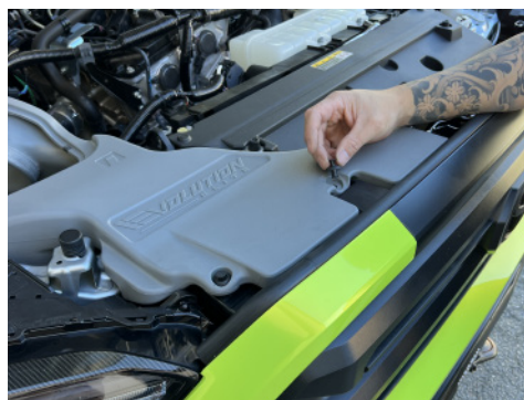
12. Using provided push pins, secure air box to radiator support.
