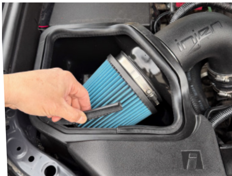
24b. Install provided rubber trim onto air box as shown and trim accordingly.
