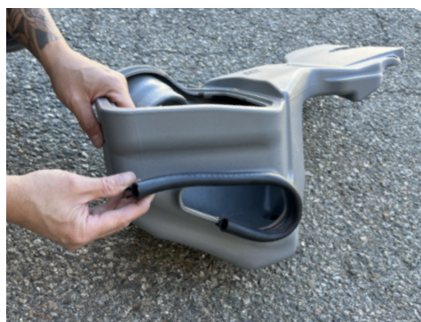
9. Install rubber bulb trim onto passenger side fender opening on EVO2201 air box.
