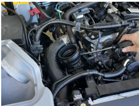
14. Install 3.50"-2.75" stepped double hump hose to turbo inlet and secure hose clamp.
