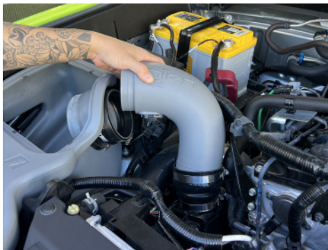
17. Install intake tube to turbo inlet hose then onto air box hose.
