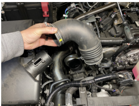
5. Loosen clamps and remove factory intake tube.
