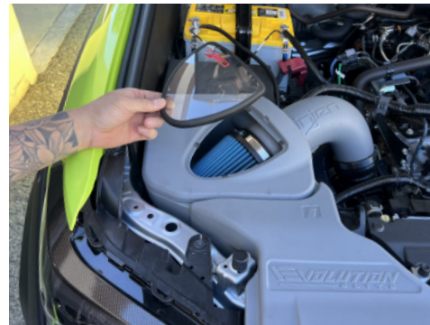
22a. Align window to lid and install.
