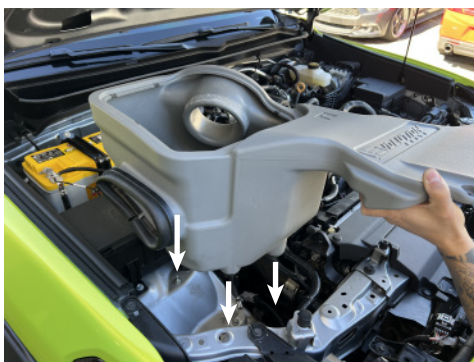
10. Align mounting grommets on EVO2201 air box to factory mounting studs.
