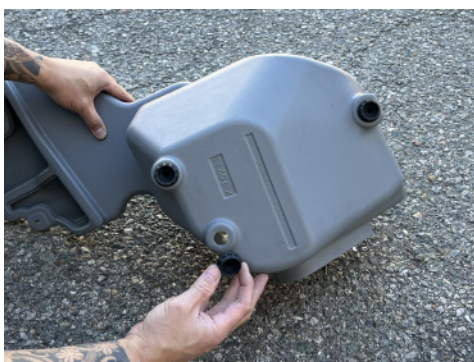
8. Install the (3) three factory mounting grommets onto EVO2201 air box.
