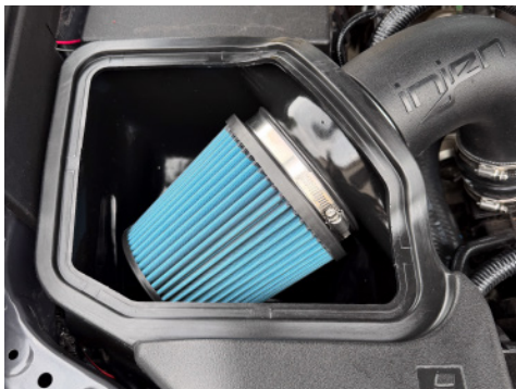
23b. The air box is now ready for the rubber trim to be installed.
