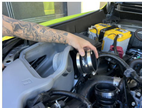
15. Install 3.75" hump hose to EVO2201 air box and secure hose clamp.
