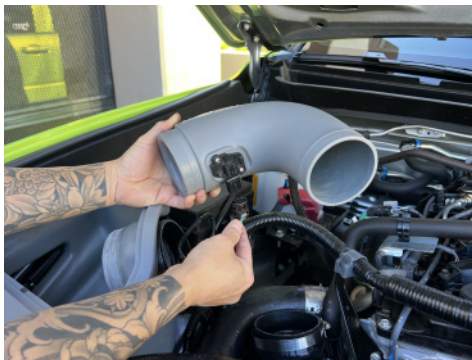
16. Reconnect the MAF sensor connector.
