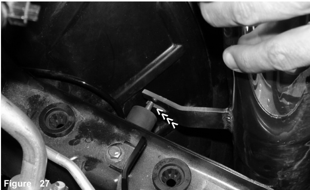
Figure 27 align and set the intake bracket over the vibra-mount stud. Press the top end of the secondary intake into the hose located on the primary intake.
