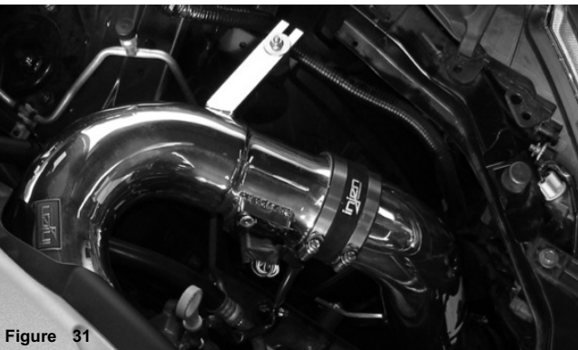
Figure 31 align the entire intake for the best possible fit. Once the entire intake has been checked and cleared for any possible rubbing or rattling, continue to tighten all nuts, bolts and clamps.
