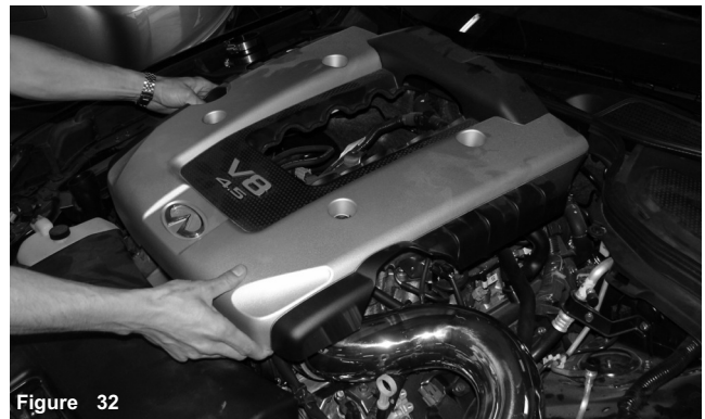
Figure 32 Once all nuts, bolts and clamps have been fastened, continue to replace the front air scoop, side cover and engine cover. Periodically, check the fitment of the entire intake system for any shifting that may cause damage.
