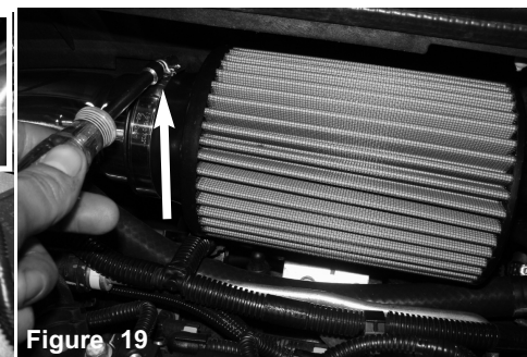
Figure 19 Install the filter to the intake tube and tighten using 8mm nut driver.
