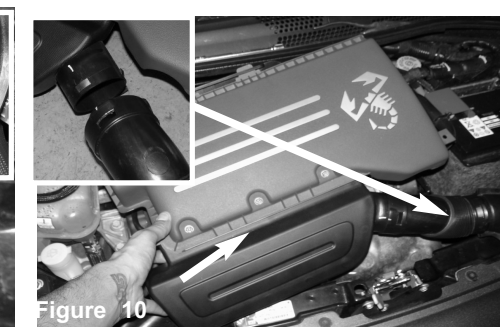
Figure 10 Now lift up and remove the air-box/engine cover from the vehicle. Disconnect the snorkel from the air box assembly.
