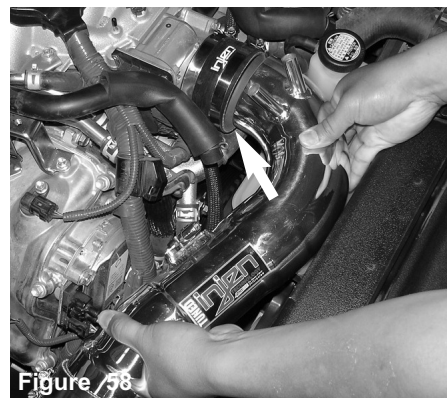
Figure 55 Secure the MAF sensor using provided M4 button head screws.
