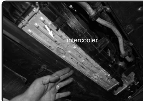
23. Re-install the intercooler into the vehicle.
