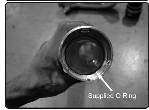
20. Install the supplied O ring into the new injen charge pipe machined flange. *Make sure the O Ring is seated properly. Note the notch on flange.* Make sure the lock clip is seated correctly.
