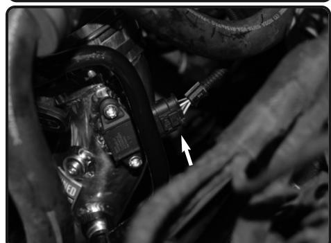
**30.** Re-connect the temperature sensor harness.
