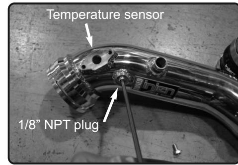
12. Install the 1/8" NPT plug to the threaded machined fitting on the charge pipe if not using.
