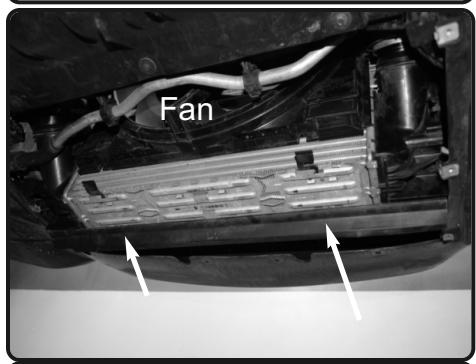
5. Carefully pull down the intercooler away from the fan.
