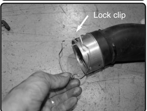
17. Carefully pull up and remove the lock clips from the plastic charge pipe.
