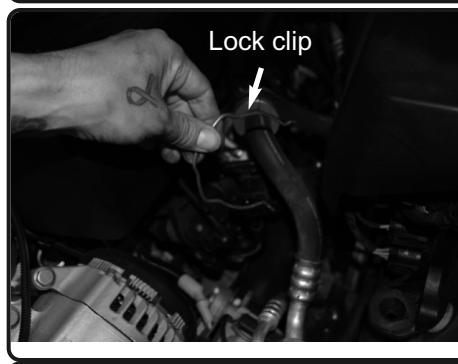
7. With pliers or flat head screwdriver, carefully pull back the lock clip on the OEM charge pipe. Save lock clip for later install.
