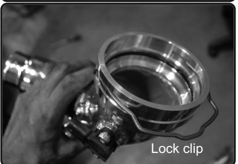
21. Re-install the lock clip from step 7 to the the new injen charge pipe machined flange.
