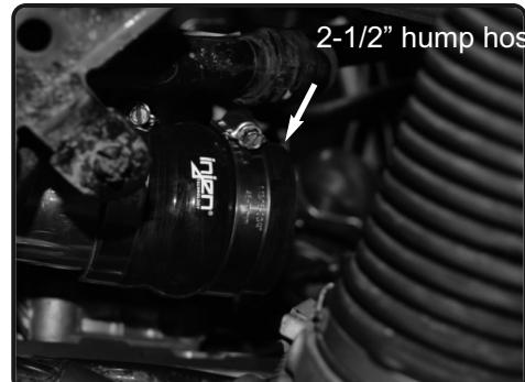
**26.** Install the 2-1/2" hump hose to the lower pipe. Tighten the clamp on the lower pipe only.
