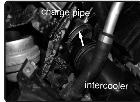
4. With flathead screwdriver, pull the clips up allowing the intercooler charge pipe to disengage on both driver and passenger side.
