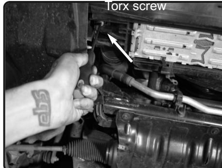
3. Loosen the 2 T25 torx bit screws holding in the intercooler on both driver and passenger side.
