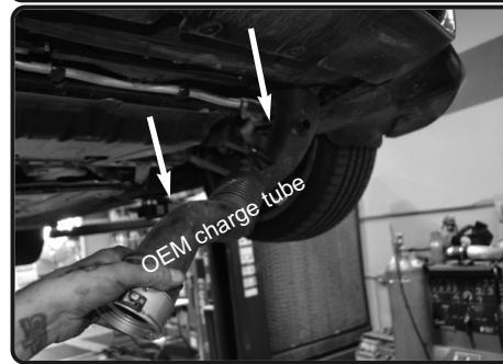
11. Rotate and remove the OEM charge pipe from the bottom of the vehicle.
