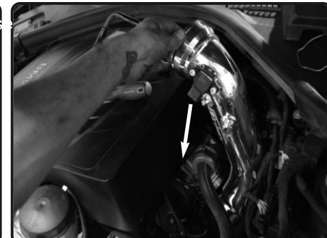
**27.** Install the upper charge pipe assembly into the vehicle and position to the lower part of the charge pipe.
