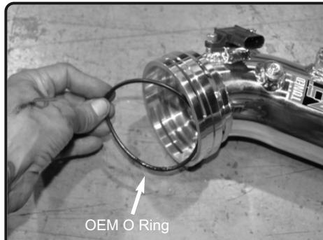
15. Now install the OEM O Ring into the new charge pipe machined fitting.
