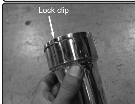
19. Re-install the lock clip from previous step to the the new injen charge pipe machined flange.
