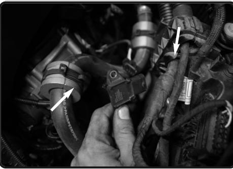
10. Loosen the 2 T25 torx screws holding in the temperature sensor and remove. This will be easier for removal of the charge pipe.
