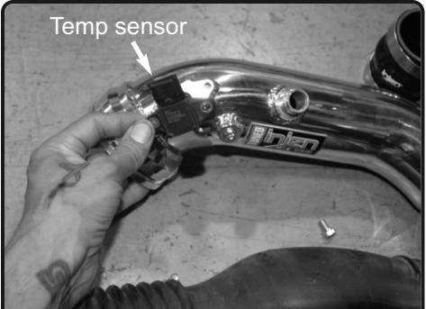
13. Install the temperature sensor into the intake tube and secure using M6 socket cap screws.
