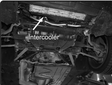
2. Place vehicle on lift. remove the undercarriage plastic guard having access to lower intercooler and pipe.
