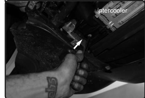
24. Secure the intercooler using the OEM screws. Re-connect the passenger side charge pipe.
