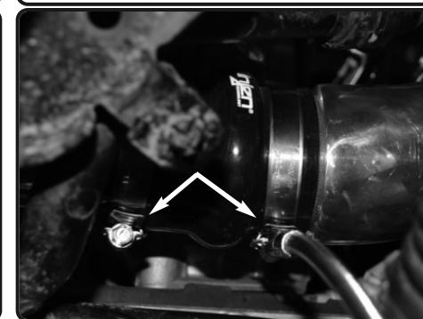
**31.** Adjust the hose and tighten all clamps using 8mm nut driver.
