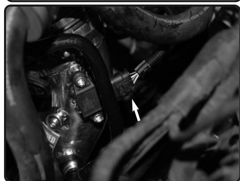
**30.** Re-connect the temperature sensor harness.
