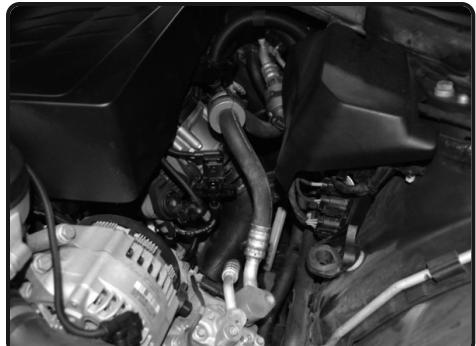
1. Stock charge pipe shown. Remove the stock intake system out of vehicle for easier installation.
