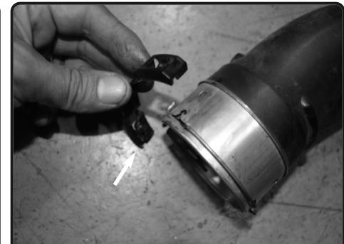
16. Pull of the plastic clip on the lower part of the plastic charge pipe.
