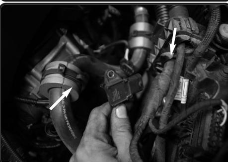
10. Loosen the 2 T25 torx screws holding in the temperature sensor and remove. This will be easier for removal of the charge pipe.
