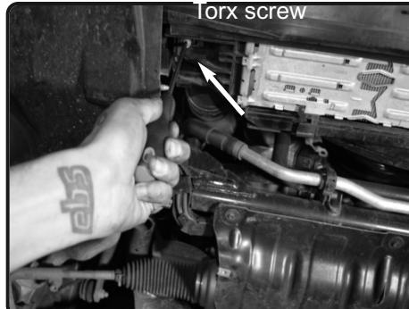
3. Loosen the 2 T25 torx bit screws holding in the intercooler on both driver and passenger side.
