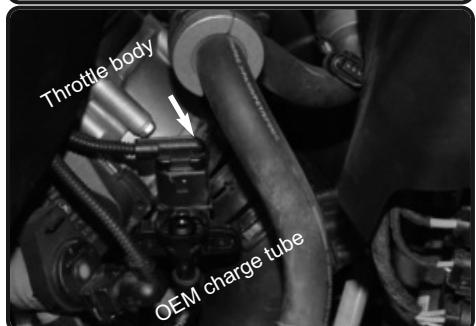
9. Pull back the charge pipe from the throttle body.
