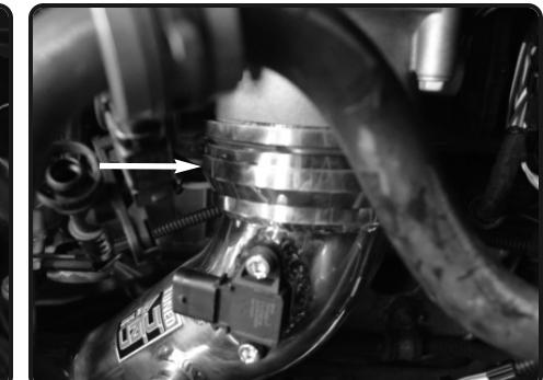
**28.** Install to the throttle body, push until you hear a click. Once seated properly, pull back and tug on pipe to make sure the flange is secured and locked.
