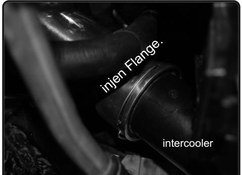
**25.** Slide the new charge pipe on the the intercooler. Locate the notch on the flange. Push until you hear a click. Once seated properly, pull back and tug on pipe to make sure the flange is secured and locked.
