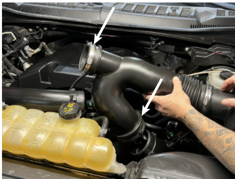
4. Loosen clamps and remove intake pipe from both turbo inlet pipes. DO NOT REMOVE ASSEMBLY. See figure 5.
