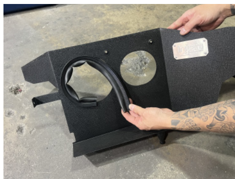
12. Install 18" rubber bulb trim (X-6058) to larger diameter hole on heat shield.
