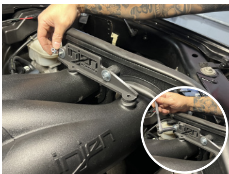
32b. Install mounting bracket onto vibramounts on heat shield using provided hardware and secure.
