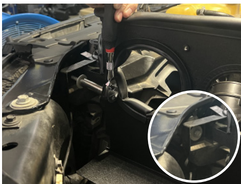
20. Using 13mm bolt from figure 10, bolt front heat shield mounting tab to factory radiator support.
