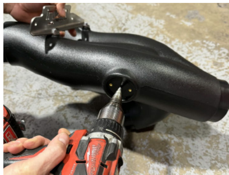
25a. Drill a 3/4" hole into the drill point located on the back of the tube where the air temp sensor mounts.
