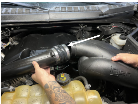
29a. Insert upper outlet of intake tube into passenger side turbo inlet pipe.
