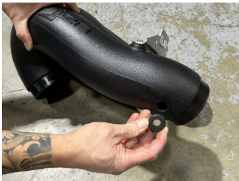
26b. Install provided air temp sensor grommet.
