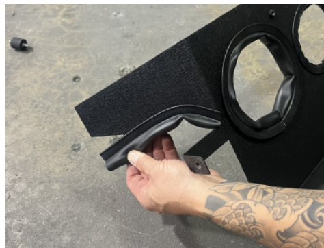
15. Install 7.5" rubber bulb trim (X-6058) to front lower portion of heat shield. Trim excess material as needed.
