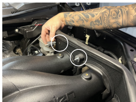
31b. Install (2) two provided vibramounts onto heat shield. **Preinstalled bracket not shown.
