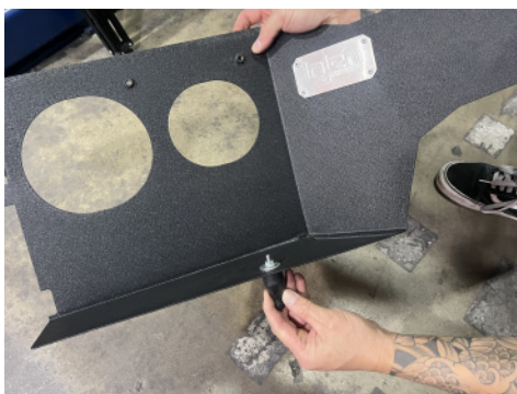
11. Install and secure provided stand-off stud through the bottom of the PF9032 heat shield using provided hardware.
