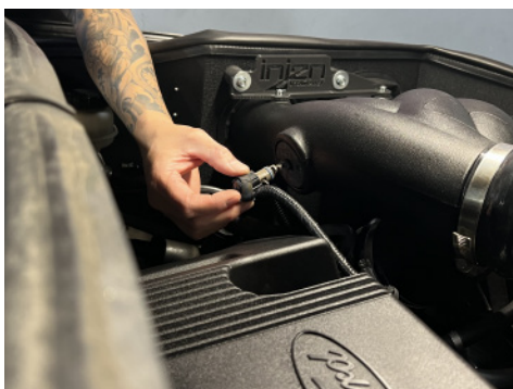
33a. Install intake air temperature sensor into back intake tube and secure.
