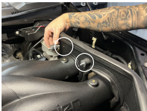
31a. Install (2) two provided vibramounts onto heat shield. **Preinstalled bracket not shown.
