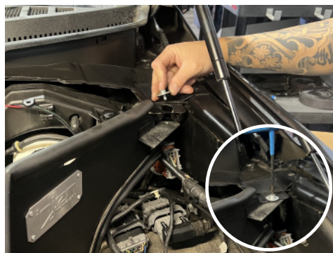
21. Bolt rear heat shield mounting tab to chassis using provided M6 hex bolt and fender washer.
