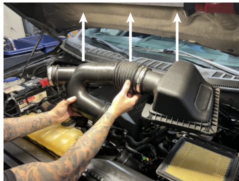
6. Unclip clamps from factory air box and remove upper air box and intake pipe assembly.
