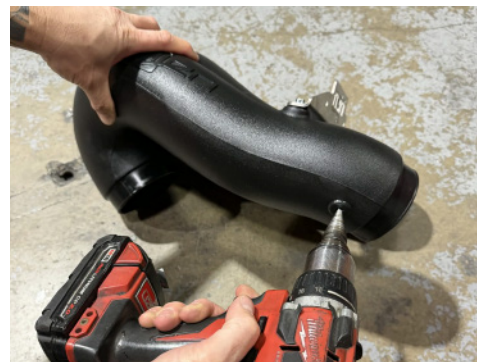
25b. Drill a 3/4" hole into the drill point located on the front of the tube.
