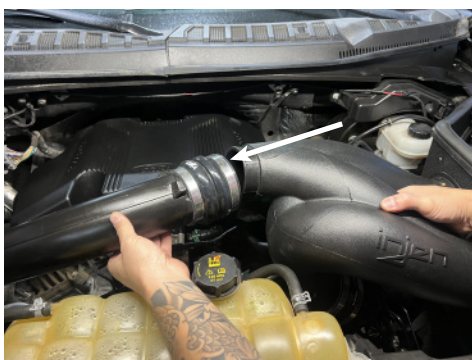
29b. Insert upper outlet of intake tube into passenger side turbo inlet pipe.
