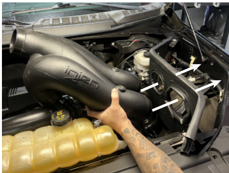
27a. Install mounting bracket onto vibramounts on heat shield using provided hardware and secure.
