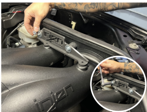
32a. Install mounting bracket onto vibramounts on heat shield using provided hardware and secure.
