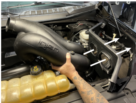
27b. Install mounting bracket onto vibramounts on heat shield using provided hardware and secure.
