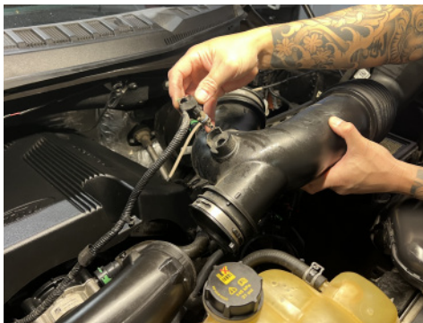
5. Remove intake air temperature sensor from factory intake pipe.
