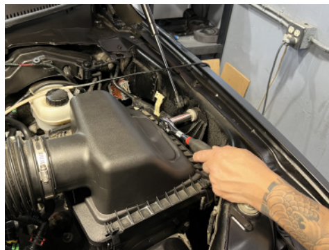
3. Unbolt 13mm bolt holding air box assembly to chassis.
