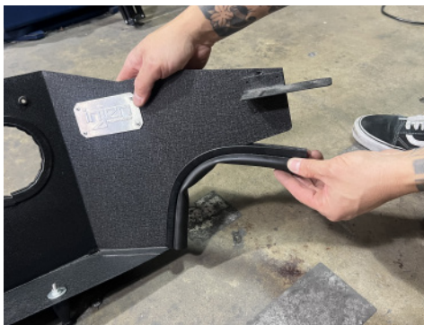
14. Install 11.5" rubber bulb trim (X-6058) to rear lower portion of heat shield. Trim excess material as needed.
