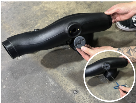
26a. Install provided air temperature sensor adapter onto intake tube using provided button head screws.
