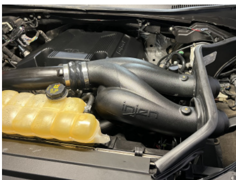
30b. Secure intake tube to both driver and passenger side turbo inlet hoses.
