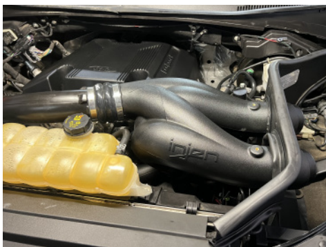
30a. Secure intake tube to both driver and passenger side turbo inlet hoses.
