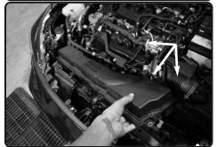
**8.** Now lift up and remove the OEM air box ram scoop.
