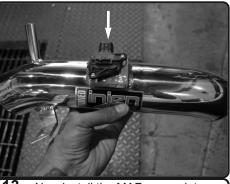
**13.** Now install the MAF sensor into the new injen tube. Secure and tighten using provided M4 screws.
