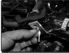
**18.** Connect the vacuum switching valve to the bracket on the intake tube. Secure using provided M5 hex screw.
