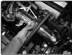
**15.** Install the intake tube assembly through the heatshield and position to the throttle body.
