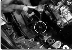
**9.** Loosen the screw on the radiator support, this will used for the heatshield.
