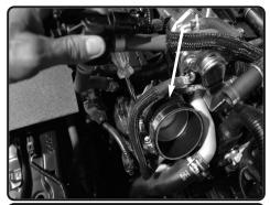
**14.** Now install the step hose to the throttle body. Tighten clamp on the throttle body only using 8mm nut driver.
