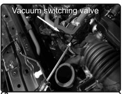
**3.** Using phillips screwdriver, loosen and remove the screw holding in the vacuum switching valve. Pull away from intake tube. Leave original bracket attached to the stock intake tube, this will not be used.
