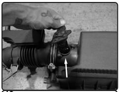
**12.** Loosen the 2 screws holding in the MAF sensor using phillips screwdriver. Carefully remove the MAF sensor out of the vehicle.
