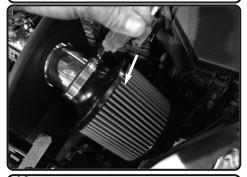
19. Install and tighten filter using 8mm nut driver.
