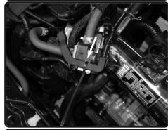
**19.** Secure harness line using provided zip tie to bracket.
