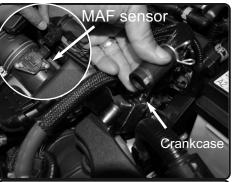
**2.** Remove the crankcase line from the stock intake tube. Disconnect the MAF sensor harness and pull harness cable from the air box.
