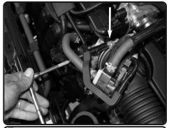
**7.** Loosen the clamp on the throttle body using 10mm socket or wrench.
