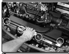
**7.** Loosen the 4 bolts holding in the OEM air box ram scoop and remove.
