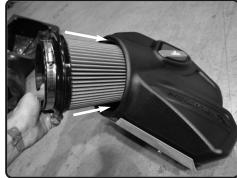
**20.** Install the twist lock filter to the inside of the air box.
