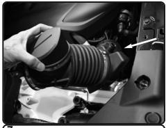
Remove the intake tube out of vehicle.
