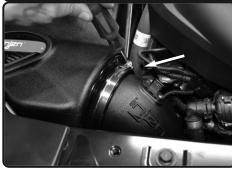
**24.** Once adjusted, tighten the clamp using 8mm nut driver.
