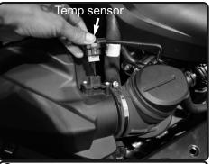
**2.** Disconnect the Temp sensor harness and pull harness cable from the air box.
