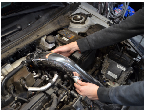
14. Next, attach the tube to the step hose.
