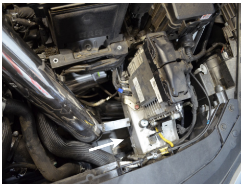
13. To install the Injen intake tube. First, route the tube below the chassis rail.
