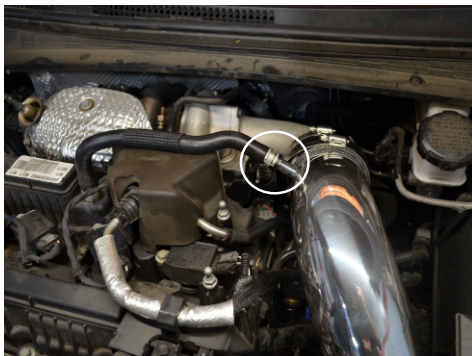
17. Reattach the crank case hose to the Injen tube, then secure the hose with the OEM tension clamp.
