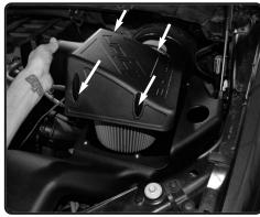
**16.** Place the plenum onto the top of the Injer lower air box. Use 4-M6X20 bolts to secure the plenum to the Injen lower air box
