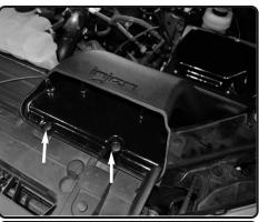
**14.** Re-use the two plastic retaining rivets from figure 2 to secure the Injen lower air box scoop to the radiator support
