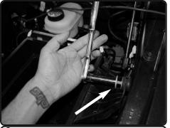
**6.** Loosen the bolt holding in the bottom of the airbox using 13mm socket or wrench.
