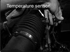
**3.** Disconnect the temperature sensor harness.
