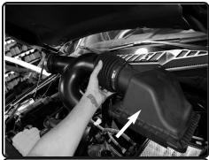
**5.** Un-clip the upper half of the air box attached to bottom of air box. Remove stock assembly out of vehicle.
