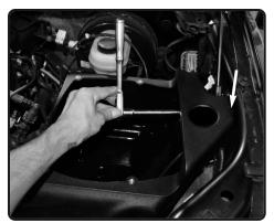
**13.** Use the OE air box bolt to secure the lower Injen air box to the chassis
