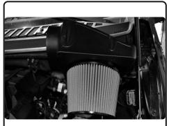
**15.** Place the filter onto the Injen plenum and connect the 3mm vacuum line from the Filter Minder to the barbed fitting on top of the filter
