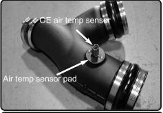
**18.** Use the supplied M4 bolts to secure the Molded air temp sensor pad onto the Injen intake pipe and then push the AIT sensor into the sensor pad and twist to secure the AIT sensor to the sensor pad
