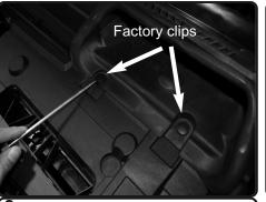
**2.** Remove the two plastic retaining rivets from the air scoop.
