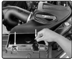
**15.** Install the provided push in rivets to the front of the scoop to the OEM holes from step 2.
