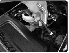
**18.** Re attach the harness to the air box holes on back side.
