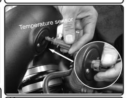
**18.** Install the temperature sensor into the adaptor. Once seated correctly turn and lock into position.
