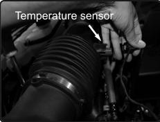
**7.** Disconnect the temperature sensor harness.
