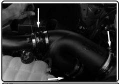
**17.** Adjust for fit, and tighten all the clamps using 8mm nut driver.
