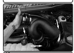
**16.** Install the intake tube assembly into the vehicle and position. Positon the intake tube into the filter and intake pipes.
