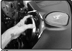
**17.** Once the filter is seated, turn the the filter in either direction a 1/4" turn.
