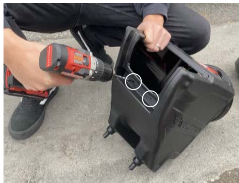
3. Drill out the two indents located on the back of the air box with a 9/32" drill bit.
