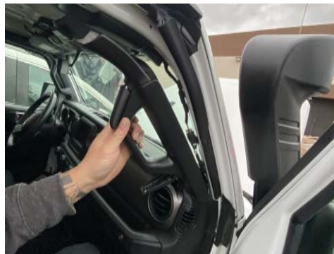
18. Pull firmly on the pillar grab handle to detach it from the pillar.
