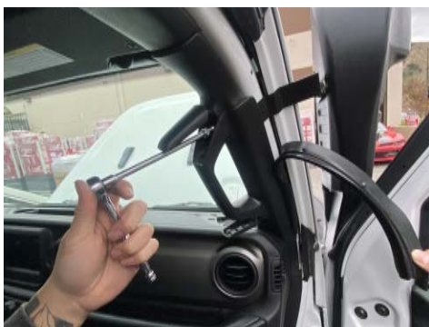
23. Reinstall the pillar grab handle with the upper bracket in place. Reinstall the speaker cover and door seal.
