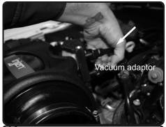
**16.** Connect the vacuum lines to the vacuum adaptor on the airbox.
