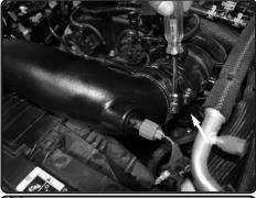
**20.** Secure and tighten all the clamps on the intake tube using 8mm nut driver.
