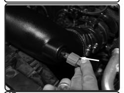
**17.** Install the air temp sensor to the rubber grommet on intake tube and reconnect the harness.
