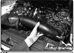
**18.** Install the provided rubber grommmet to the intake tube hole. Insert the Injen intake tube into the vehicle. Position tube to the filter and turbo inlet. Postion for best fit.
