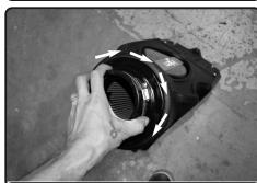
**12.** Once the twist lock filter is seated properly, rotate the filter in either direction a 1/4" turn untill filter locks into place.
