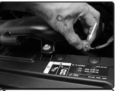
**2.** Carefully disconnect the temperature sensor, pull back the harness from the intake tube.
