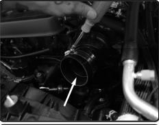
**8.** Install the provided step hump hose to the throttle body. Secure using provided clamps.
