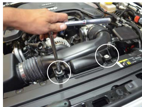
3. Remove the 2 bolts holding in the intake tube.
