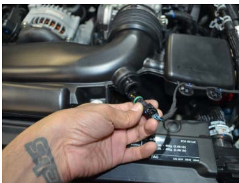
2. Twist the IAT sensor then carefully remove the sensor from the intake tube.
