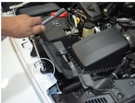
4. Remove the bolt holding in the airbox. Save for later install along with the grommet and crush washer.
