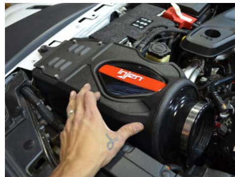
15. Line up the airbox to the factory grommet and push down. Secure the airbox using the OEM screw from step 4.
