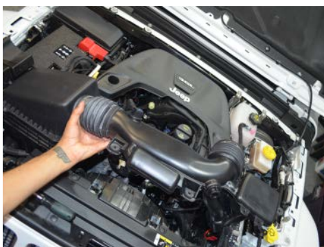
7. Remove the stock intake system out of the vehicle.
