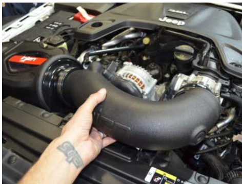
17. Insert the Injen intake tube into the vehicle. Position tube to the filter and step hose.
