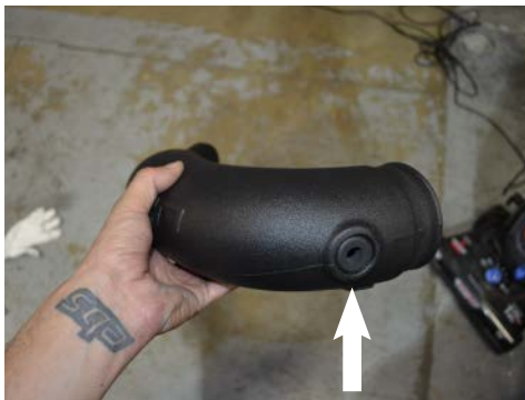
16. Install the provided rubber grommet to the intake tube
