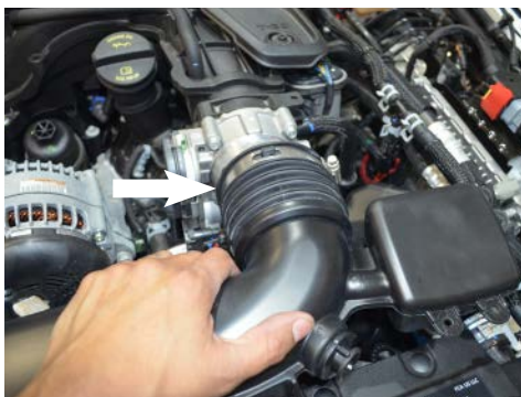
5. Loosen the clamp on the throttle body and pull back the intake tube from the throttle body.
