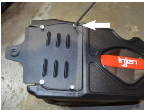
13. Secure the bracket to the air box using M6 socket cap screws.
