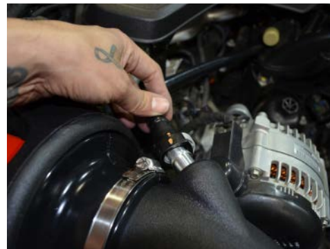
18. Connect the crank case vent tube to the machined fitting on the intake tube.
