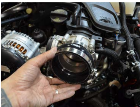
11. Install the provided step hump hose to the throttle body. Secure using provided clamps.
