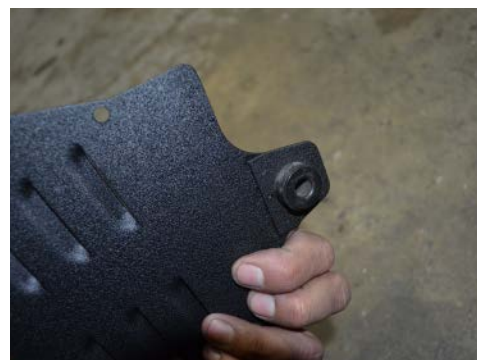
12. From step 4, install the grommet with crush washer to the hole on the airbox bracket.
