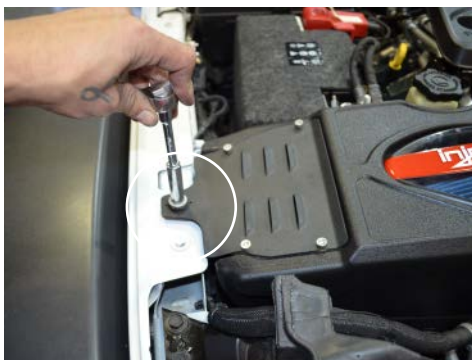
20. Tighten the bracket using the oem bolt from step 4.
