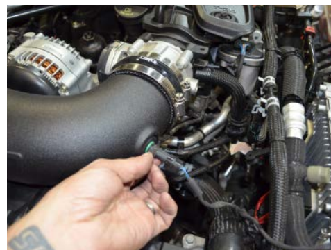
22. Install the IAT sensor to the rubber grommet on intake tube and reconnect the harness.
