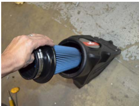
14. Install the twist lock filter on to the Injen air box. Once seated, rotate the filter a 1/4 turn in either direction so the filter can lock into place.
