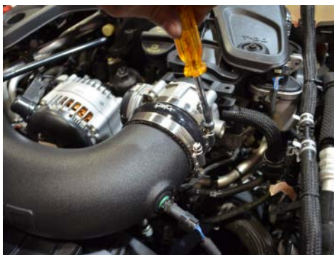
21. Secure and tighten all the clamps on the intake tube using 8mm nut driver.
