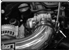
**22.** Position the intake for best fit. Tighten the clamp with an 8mm nut driver.
