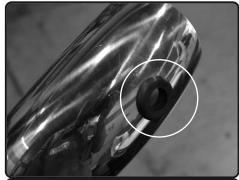
**20.** Install the provided grommet to the hole on the intake tube.
