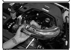
**21.** Install the intake tube to the vehicle. Position to the hose and filter.
