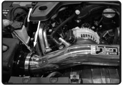
**23.** Tighten the clamp on the filter using an 8mm nut driver.
