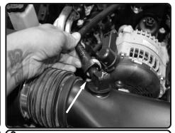
**3.** Pull back crank case line from air box fitting.
