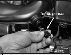
**2.** Disconnect the Temperature sensor harness.
