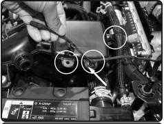
**4.** Pull back the temperature sensor harness from the intake tube.
