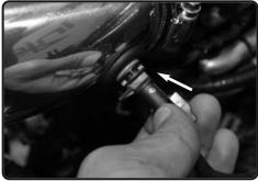
**24.** Reinstall the temperature sensor to the grommet on the intake tube.
