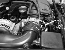
**6.** Loosen the clamp on the throttle body using an 8mm nut driver.
