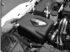
**18.** Powerflow box installed and seated properly.
