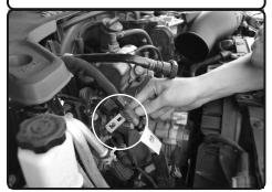
**9.** eTORQUE MODELS ONLY: Remove the nut holding down the generator harness and remove the harness from the bracket.
