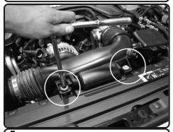
**5.** Loosen the 2 bolts holding in the intake tube using 10mm socket or ratchet.
