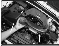
**8.** Now lift up and remove the air box assembly out of the vehicle.
