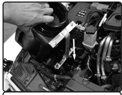
**16.** Install the powerflow box assembly into the vehicle.
