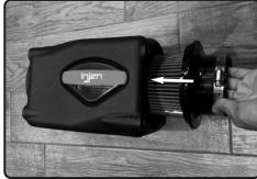
**12.** Install air filter to the powerflow box.
