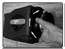
**13.** 1)Insert twist lock filter to the air box. 2)Once seated, rotate in either direction 1/4 turn till filter locks.
