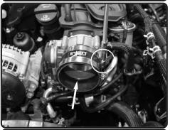
**19.** Now install the straight hose with clamps provided to the throttle body.
