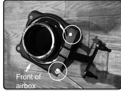
**15.** Install the provided Bracket to the powerflow box using provided M6 screws. Secure and tighten.
