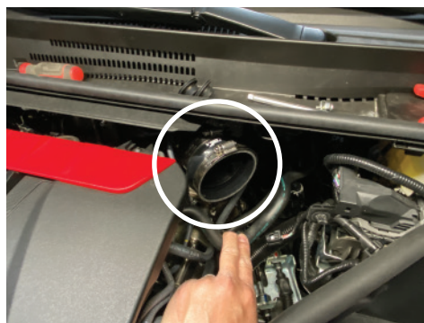
23. Place the 3.125"-3.50" Step hose, #48 & #56 clamp onto the turbo inlet and secure only the #48 clamp on the turbo inlet side for now.
