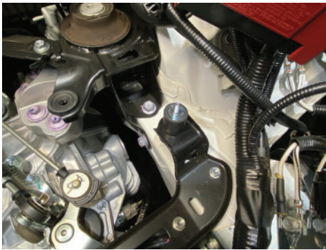
13. The 1/4" washers will be smashed in between the bracket and vibra-mount
