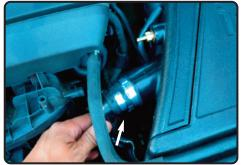
**23.** Connect the OEM air pump fitting to the machined fitting on intake plenum. If not equipped with air pump, use supplied air pump cap.
