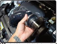
**18.** Install the molded turbo hose with clamps to the MAF sensor. Make sure the MAF sensor is in the corret direction. Note: Arrow on MAF sensor goes towards turbo.
