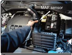
Disconnect the MAF sensor. Now lift up OEM intake air box assembly out of vehicle.
