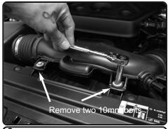
**3.** Loosen the 2 bolts holding in the intake tube and remove.
