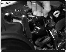
17. Make sure the harness on the vacuum lines are secured and you hear the click. Tug and pull back to verify the're connected.
