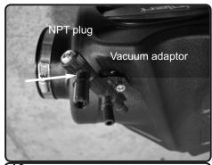
**13.** Attach the Vacuum adaptor to the insert to the side of the airbox using supplied allen screw. Secure the top of the vacuum adaptor using supplied NPT Plug.
