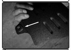
**9.** From step 4, install the grommet with crush washer to the hole on the airbox bracket cover.
