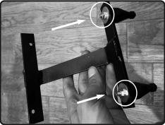
**14.** Install the provided stand off studs to the bracket and secure using fender washers and nuts. Secure and tighten.
