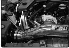
**23.** Tighten the clamp on the filter using an 8mm nut driver.
