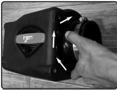
**13. 1)**Insert twist lock filter to the air box. **2)**Once seated, rotate in either direction 1/4 turn till filter locks.
