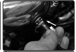
**24.** Reinstall the temperature sensor to the grommet on the intake tube.
