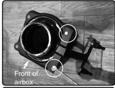
**15.** Install the provided Bracket to the powerflow box using provided M6 screws. Secure and tighten.
