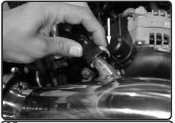
**25.** Reconnect the crank line to the intake tube fitting. Make sure you hear the click.
