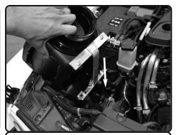
**16.** Install the powerflow box assembly into the vehicle.
