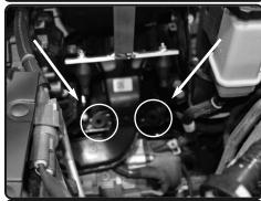
**17.** Make sure the stand off studs are seated in the OEM grommets properly.
