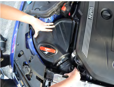
19. Press the Injen tube into the twist lock filter.
