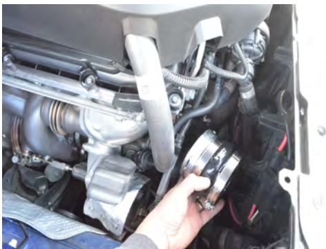
10. Press the 3.50" Hump hose on to the billet machine adapter then secure it using the provide clamps.
