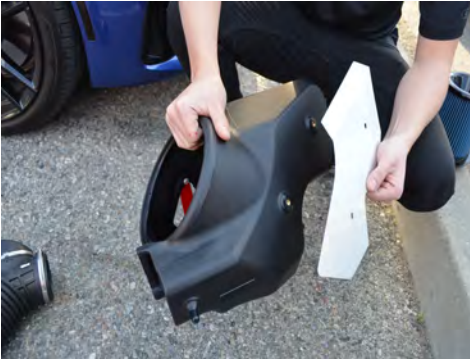
16. Bolt down the provided heat shield to the Injen air box.
