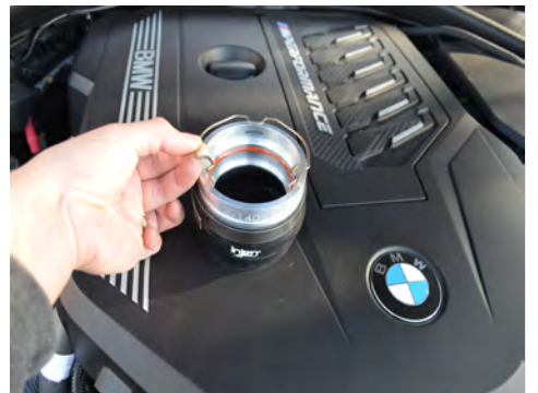
9. Install the factory retaining clip on to the billet machined adapter. The center of the retaining clip must face the part number.
