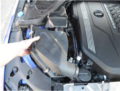
4. Remove the OEM air box.
