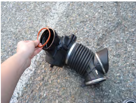
7. Take note of which direction the O-ring is installed in the OEM tube then remove the O-ring.
