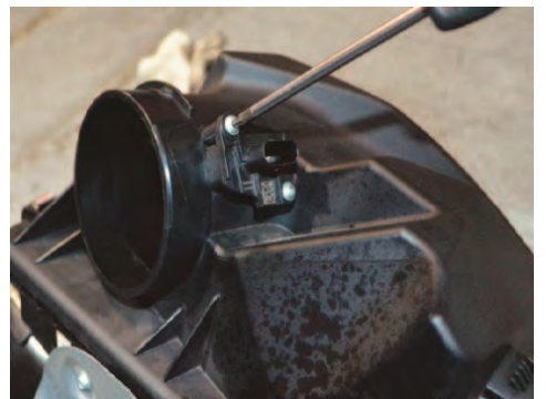
12. Remove the two screws holding the temp sensor then remove the temp sensor.
