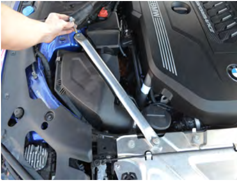
1. Remove the two bolts holding the strut tower brace. Then remove the strut tower brace.
