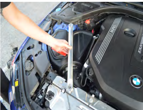
22. Reinstall the strut tower brace.
