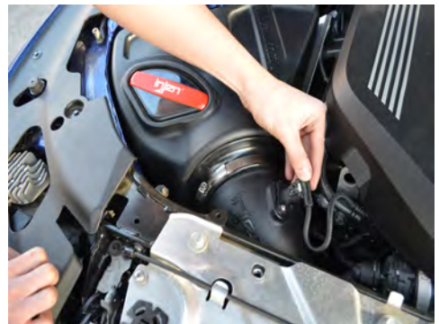
21. Plug in the temp sensor haarness.
