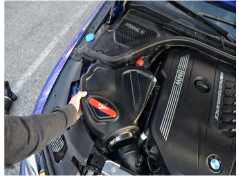
16. Install the Injen air box into the engine bay. Line up the studs on the air box to the factory grommets and press down on the box.
