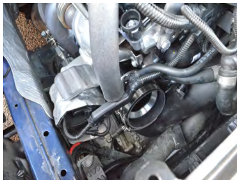
11. Press the billet machined adapter on to the turbo inlet until you hear the retaining clip snap into place.
