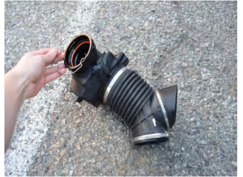
6. Remove the OEM retaining clip from the tube. It will be reused on the Injen intake.
