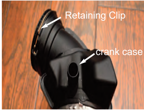
5. To remove the OEM tube, pull back the retaining clip on the tube with a prying tool. Next, slide out the tube from the turbo. Finally, press on the tabs located on the crank case line and detach it from the tube.
