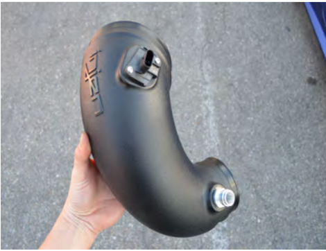
13. Install the temp sensor onto the Injen tube and secure using the provided M4 button head screws.
