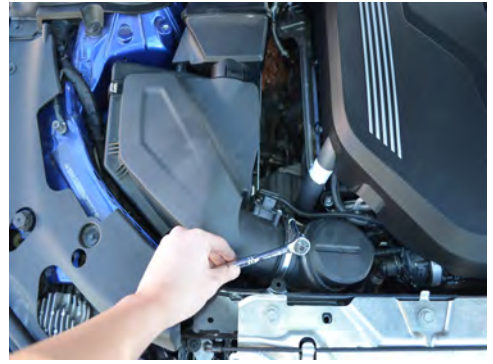
3. Loosen the clamp holding the OEM air box and tube together.
