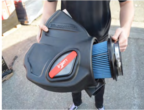
17. Install the twist lock filter on to the Injen air box. Once seated, rotate the filter a 1/4 turn in either direction so the filter can lock into place.
