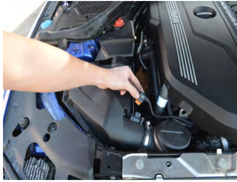
2. Disconnect the temp sensor harness.
