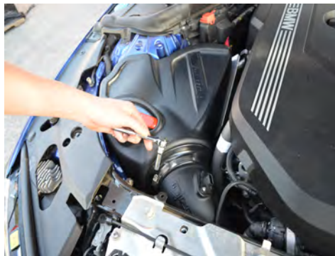
20. Secure the clamp on the twist lock filter.
