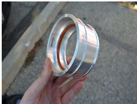
8. Install the O-ring onto the billet machined adapter. Make sure to install it in the same direction as the OEM tube.
