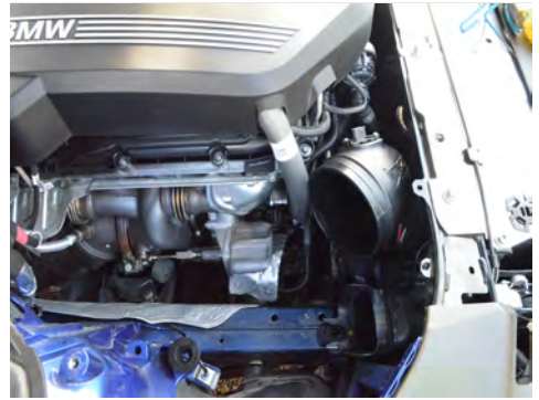
15. Secure both clamps on the 3.50" hump hose.
