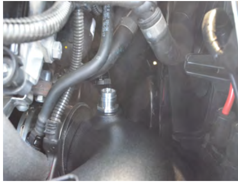
14. Install the Injen tube and attach the crank case line to the machined fitting.
