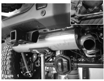
Remove the stock muffler using 15mm socket and wrench. Remove the hangars from stock isolators. Install the new Injen Axle Back Exhaust. Position the hangars to the stock isolators. Use Provided #66 torsion clamp in the kit. Position for the best to have access to the 17mm nut on clamp. **Do not tighten.** Install the Black tips to the exhaust adjust and fit to desired position and tighten.
