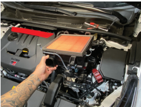
7. Lift up and remove the lower portion of the OEM air box assembly
