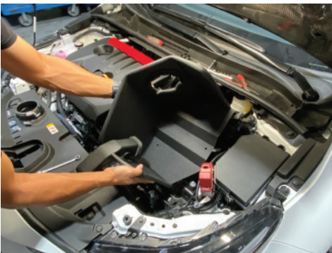
19. Lower the heat shield into the engine bay and align the studs on the vibra mount from figures 14 and 17.
