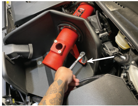
26. Use a M6 nut and fender washer to secure the intake bracket to the vibra-mount
