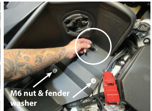
21. Place the male/female vibra mount onto the rear vibra-mount from figure 17 & then place a M6 nut and fender washer onto the front vibra-mounts in figure 14
