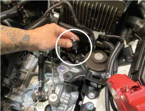
16. Place a male/male vibra-mount after removing the 10mm bolt from figure 15
