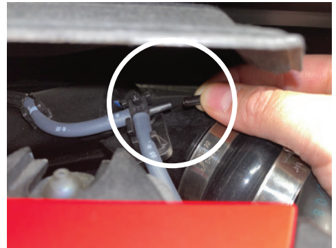
6. Place the supplied 3mm vacuum cap onto the T-fitting
