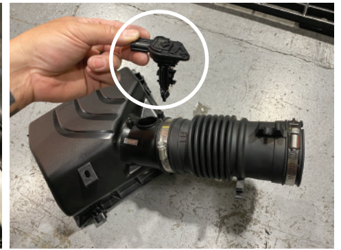
27. Remove the OEM MAF sensor from the OEM air box assembly
