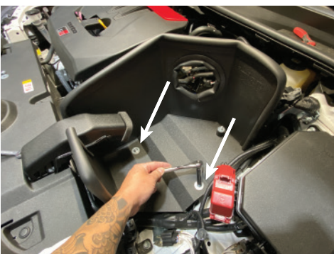
22. Secure the two M6 nuts from figure 21
