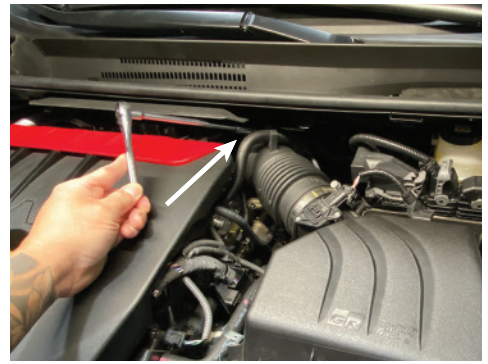
3. Loosen the clamp on the intake tube
