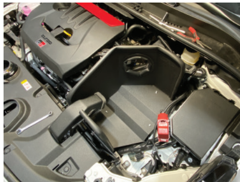
20. Heat shield shown correctly mounted to vibra-mounts
