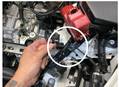
9. Use the supplied zip tie and secure the vacuum switching valve to the battery cables. Reattach the harness from Figure 1
