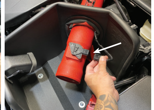
30. Run the MAF sensor harness through the heat shield and then reconnect the MAF sensor harness to the MAF sensor
