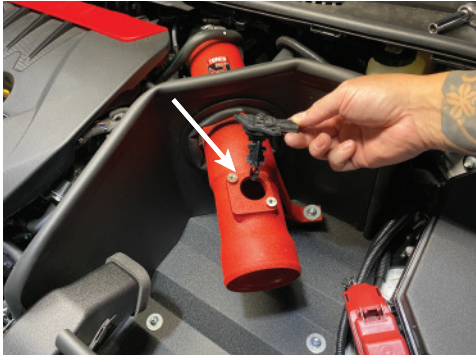
28. Place the OEM MAF sensor into the Injen MAF adapter
