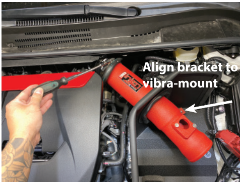
25. Align the bracket onto the rear vibra-mount and then secure the #56 clamp once the intake pipe has been adjusted for best fitment.
