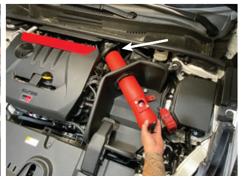
24. Insert the intake pipe through the heat shield hole and slip the tube into the 3.125"-3.50" Step hose.
