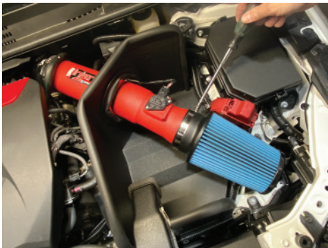
31. Place the filter onto the end of the pipe and then secure the clamp
