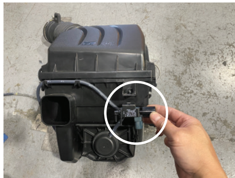
8. Remove the vacuum switching valve from the OEM air box assembly
