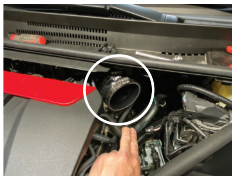
23. Place the 3.125"-3.50" Step hose, #48 & #56 clamp onto the turbo inlet and secure only the #48 clamp on the turbo inlet side for now.
