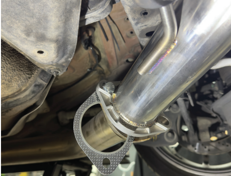
4. Insert the injen front pipe hanger into the rubber insulator, then secure the front pipe to the oem exhaust with the provided hardware. Ensure to use the provided exhasut gasket.
