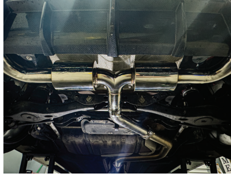
5. Insert the muffler section hangers into the rubber insulators, then secure the muffler section to the front pipe with the provided clamp.
