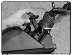
**13.** Loosen and remove the MAF sen-sor from the factory air box.
