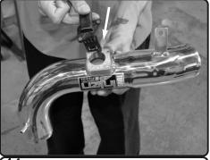
**14.** Install the MAF sensor into the new intake tube.
