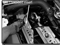
**8.** Install the M8 vibramount to the thredded insert on frame. Secure and tighten.
