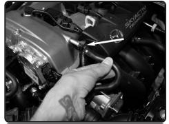
**3.** Pull out crank case line from engine fitting.
