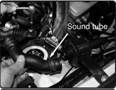
**4.** With pliers, bull back the line from sound tube. Loosen the 10mm screw holding in the sound tube.
