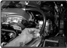
**22.** Now connect the provided 10mm hose to the engine fitting and intake tube.
