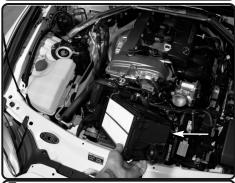
**7.** Now carefully remove the bottom air box assembly by pulling up from vehicle.
