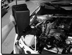
**6.** Carefully lift up and remove the upper stock air box assembly.
