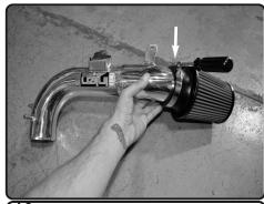
**16.** Now install the air filter to the tube and tighten using 8mm nut driver.
