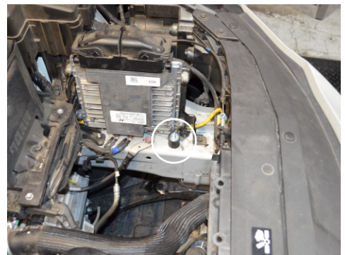
12. Fasten the provided vibra mount onto the threaded hole on the chassis.
