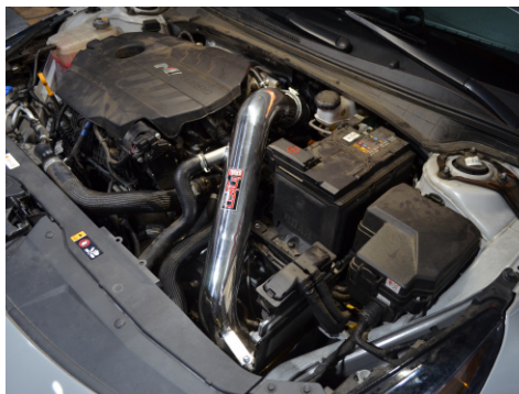
24. Ensure that all bolts, clamps and hoses are properly secured.
