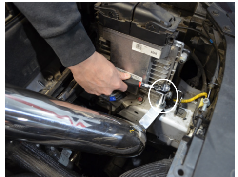
15. Line up the bracket to the vibra mount, then secure the bracket with the provided M6 nut and washer.
