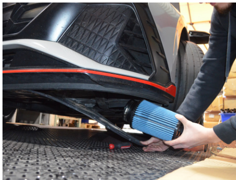
21. Pull down the under cover, then insert the air filter through the bottom front bumper.
