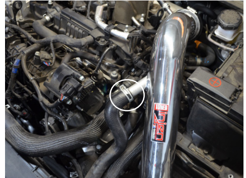
18. Reattach the diverter valve hose to the injen tube, then secure the hose with the OEM tension clamp.
