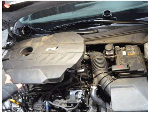
2. Remove the engine cover by firmly lifting it on all four sides.
