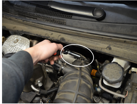
5. Loosen the clamp securing the OEM tube to the turbo inlet, then detach the tube.
