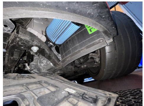
22. Secure the air filter to the intake tube with the provided clamp, then reattach the under cover.
