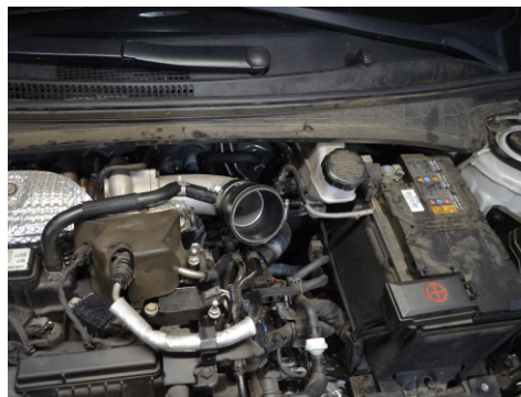
11. Place the provided step hose on to the turbo inlet. Only secure the clamp on the turbo inlet for now.
