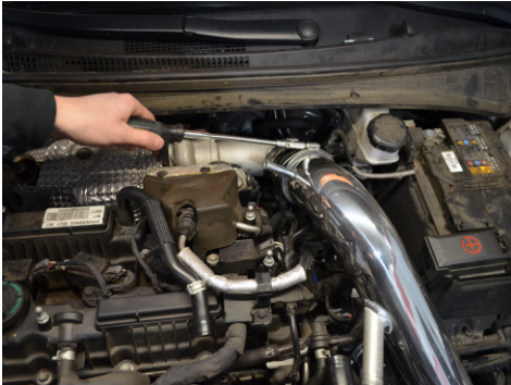
16. Ensure there is enough clearance between the tube and battery terminal, then secure the clamps on the step hose.
