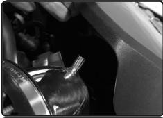
**23.** Re-install the radiator cover. **Note:** fitting on intake tube is for grommet on radiator cover to seat and secure.
