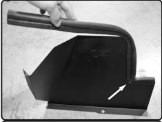
**6.** Install rubber trim to the top of the heatshield. Notch corner for easier installation.
