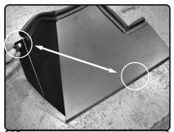
**12.** Install the provided grommets to the holes in the heatshield.
