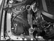
**5.** Locate the 2 threaded studs in the engine compartment, this will be used for the heat shield
