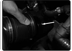
7. Loosen the clamp on air box and pull back the intake tube.
