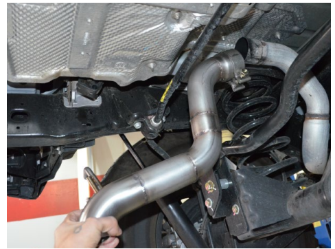
3. Attach the muffler delete pipe to the OEM midpipe. Insert the hanger into the rubber insulator.
