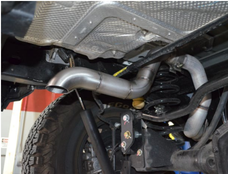
4. Secure the muffler delete pipe using the provided clamp.
