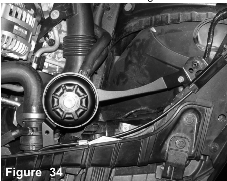
Figure 34 Install the reservoir into the cup and secure. Note: Make sure the reservoir bottle sits all the way down and tight.
