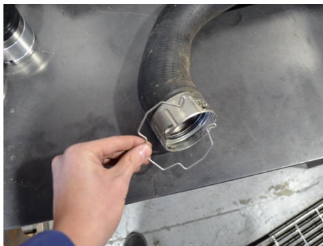
23. Remove the C-Clip from both intercooler hoses.
