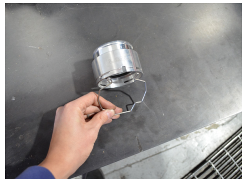
24. Install the C-Clip onto both machined adapters.
