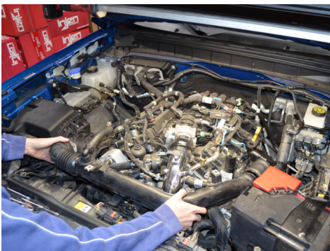
34. Reinstall the intake tube.
