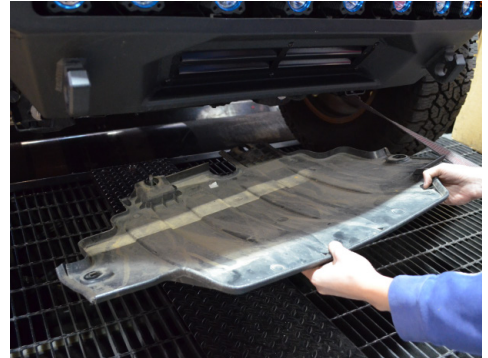
18. Remove the OEM skid plate.
