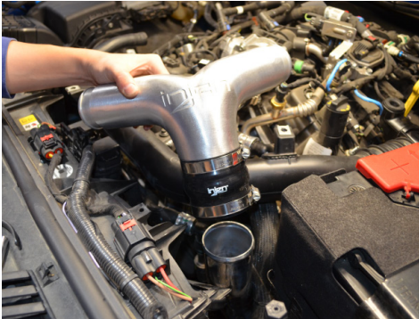
40. Attach the 2.75" hump hose to the cast Y-Pipe. Then secure the Y-Pipe to the primary hot side charge pipe.
