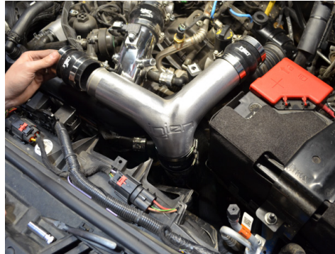
41. Attach the 2.25" hump hose to both ends of the cast Y-Pipe. Secure using the provided clamps.
