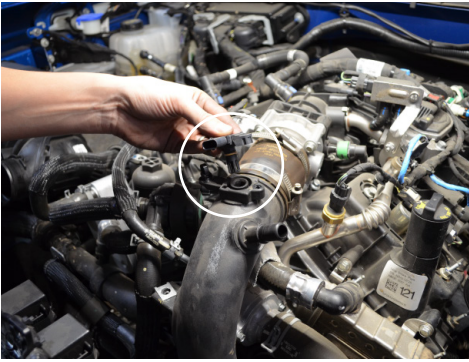
13. Remove the pressure sensor from the cold side intercooler pipe.
