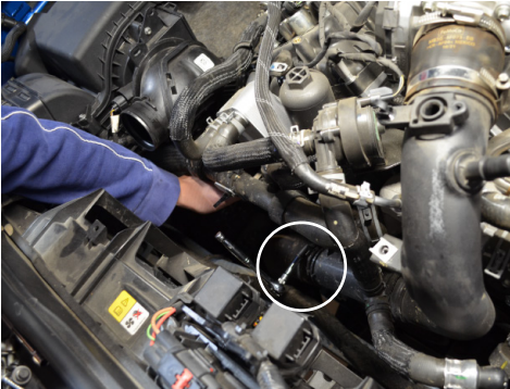
16. Loosen the clamp securing the plastic intercooler pipe to the intercooler hose.
