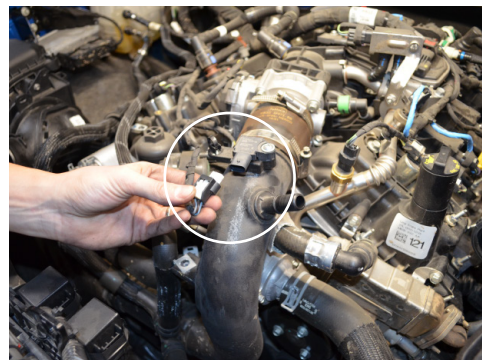
12. Disconnect the pressure sensor harness.
