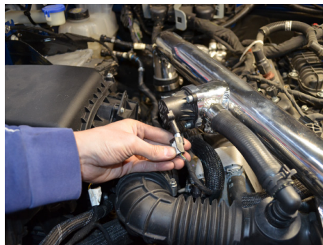
47. Reconnect the diverter valve harness.
