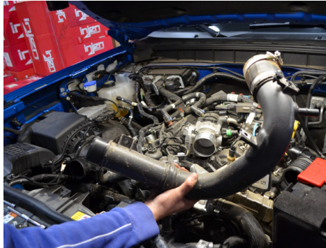
17. Remove the intercooler pipe from the engine bay.
