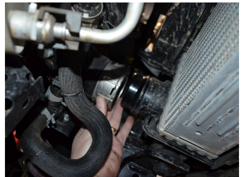
21. Disengage the C-Clip securing the hot side (driver side) hose then detach the hose from the intercooler.
