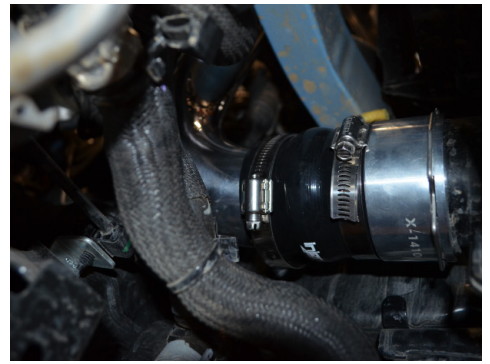
39. Secure the primary hot side intercooler pipe. Note: Make sure the pipe from fig. 38 does not come in contact with A/C compressor.
