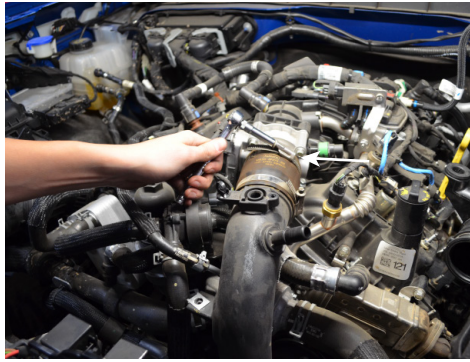
14. Loosen the clamp securing the cold side intercooler pipe to the throttle body.
