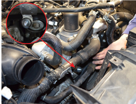
29. Secure the provided vibra-mount to intercooler pipe bracket using the provided M6 nut and washer.
